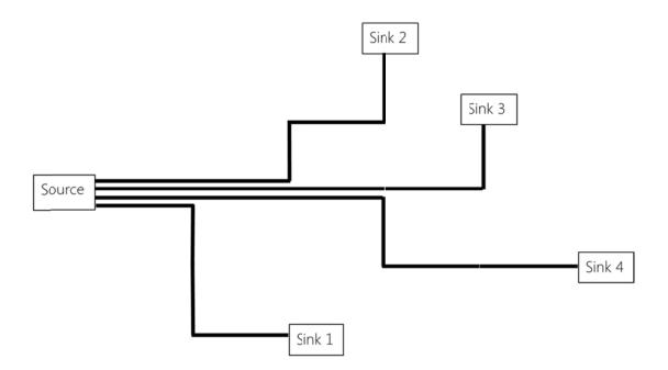
Figure 21. An unmerged pipeline connectivity demonstration for a given water source, distributing water to several nearby water sinks
