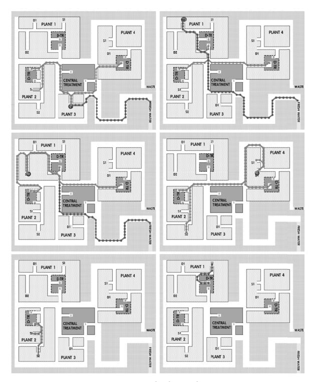
Figure 39. Backward pipeline branching with 90°, 45° and 135° pipe bending illustrated (Case 4)
