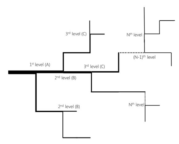
Figure 25. Node level illustration (for both forward and backward branching)
