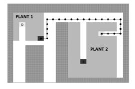
(a) Type 1 connectivity from Plant 1 Source to Plant 2 Sink, through service corridor area
