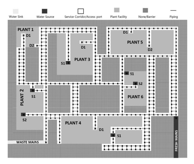
Figure 6. Industrial City Case Study Layout, with Type 1 connectivity mesh illustrated
