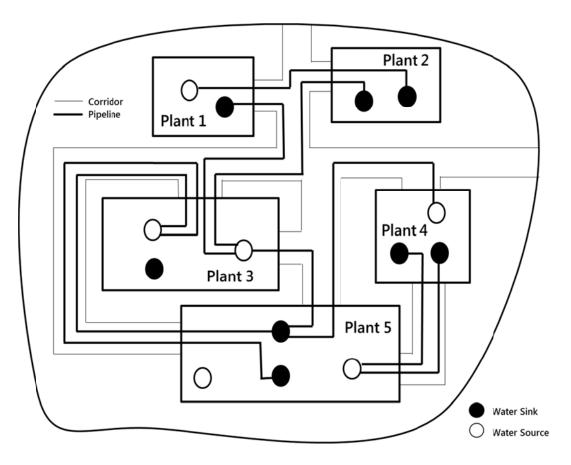
Figure 20. Typical output of a source-sink mapping activity, for the design of interplant water networks
