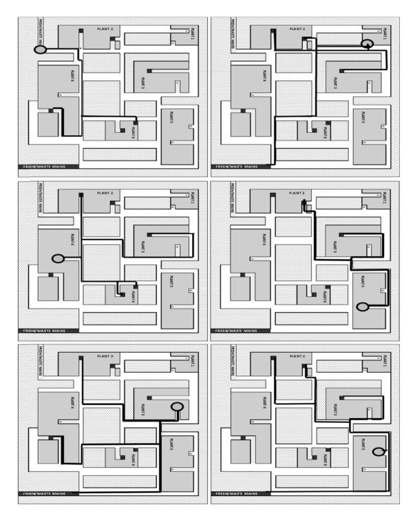
Figure 33. Case 3 interplant piping illustrated after merging, via backward branching
