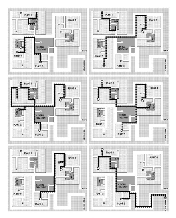
Figure 36. Forward pipeline branching with  $90^0$  pipe bending illustrated (Case 1)
