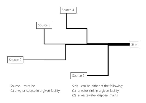
Figure 24. A merged pipeline connectivity demonstration via backward branching, for a given water sink, receiving water from several nearby water sources
