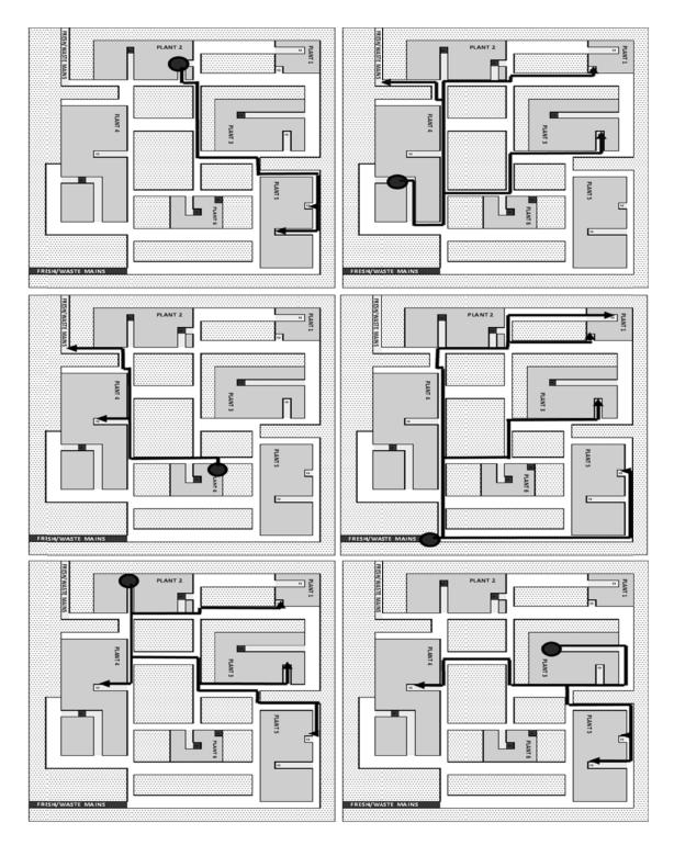
Figure 31. Case 1 interplant piping illustrated after merging, via forward branching
