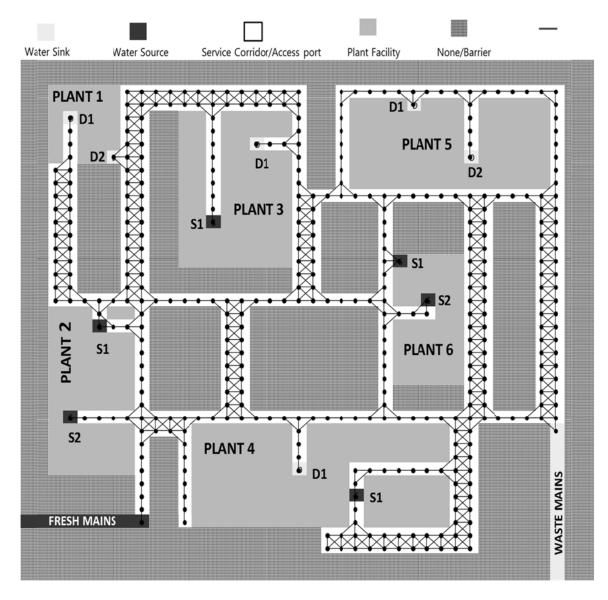
Figure 7. Industrial City Layout (Fresh and Waste mains positioning switched), with Type 2 connectivity mesh illustrated
