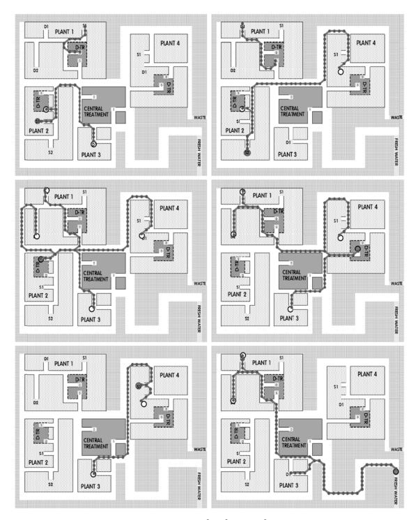
Figure 37. Forward pipeline branching with  $90^{\circ}$ ,  $45^{\circ}$  and  $135^{\circ}$  pipe bending illustrated (Case 2)
