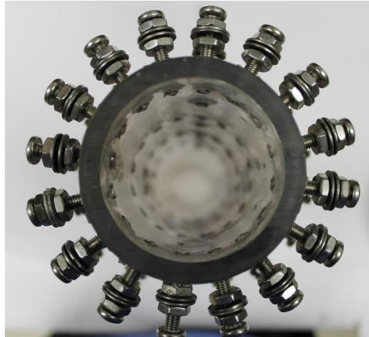
Figure 13: Cross-sectional view of the pipe showing the electrodes arranged in circular pattern
