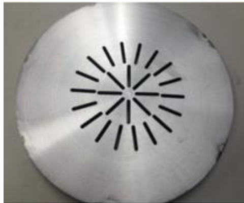
Figure 2: Slotted Orifice Plate
