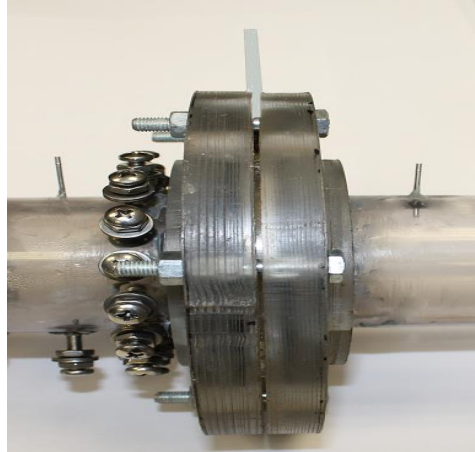
Figure 16: Pressure taps inserted upstream and downstream of the orifice plate
