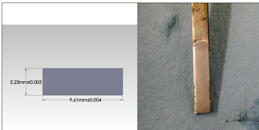
Fig. 3.1 Zircaloy-4 Material. (Left) Dimensions. (Right) Post Charging.
