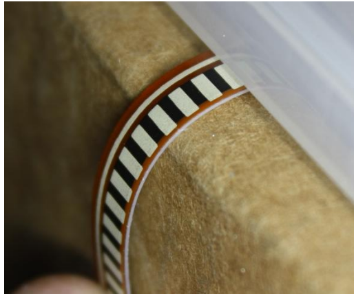
Figure 3.4 Flex sensor bent 90°
