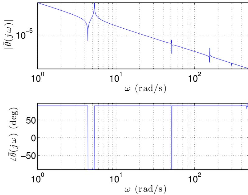
Figure 3.8: Bode Plot  $\bar{\theta}$  at  $x = 4$  ft, [76]
