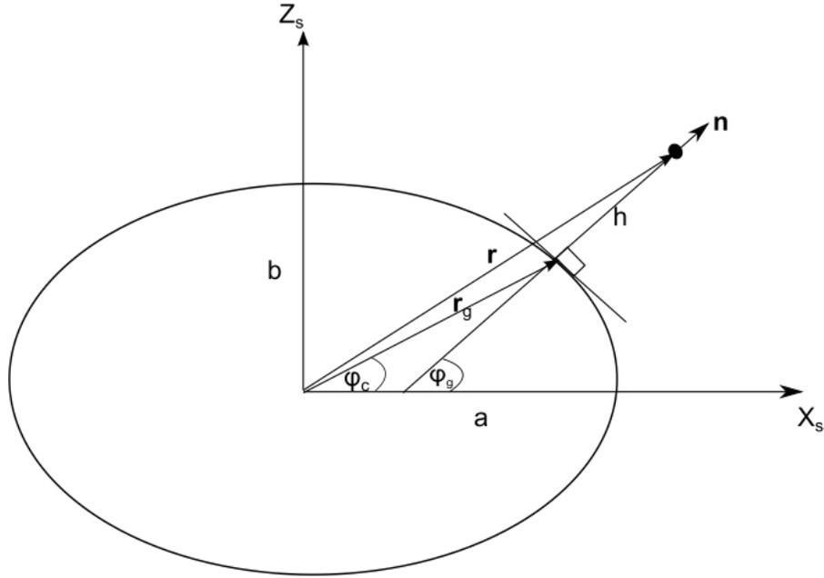
Figure 2.22: Geodetic Vs. Geocentric Latitude, [30]
