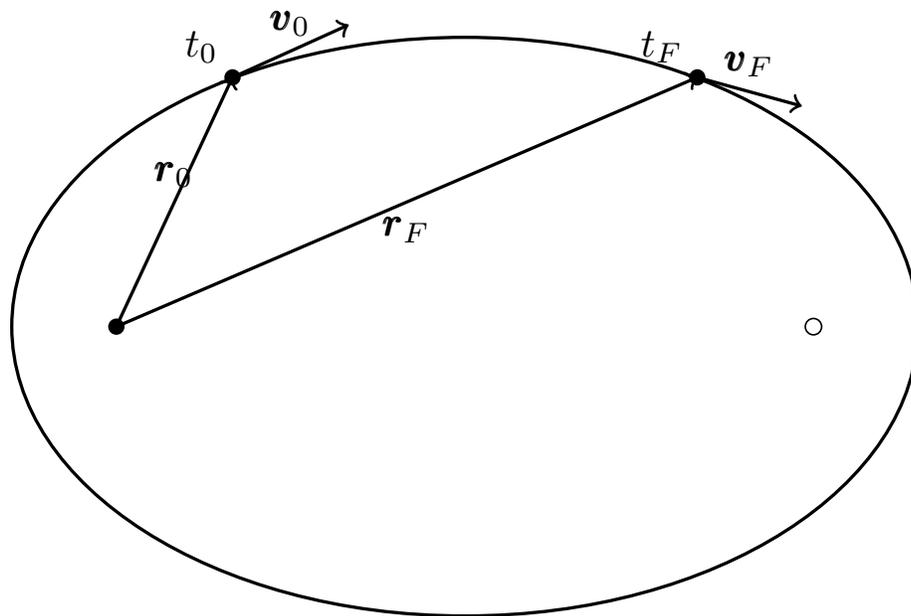
Figure 5.19: Illustration of the Orbital Transfer Problem, [123]
