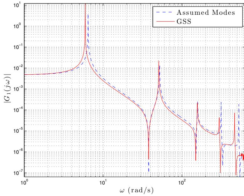
Figure 3.5: Frequency Response Comparison Tip Mass Model at  $x = 2$  ft, [76]
