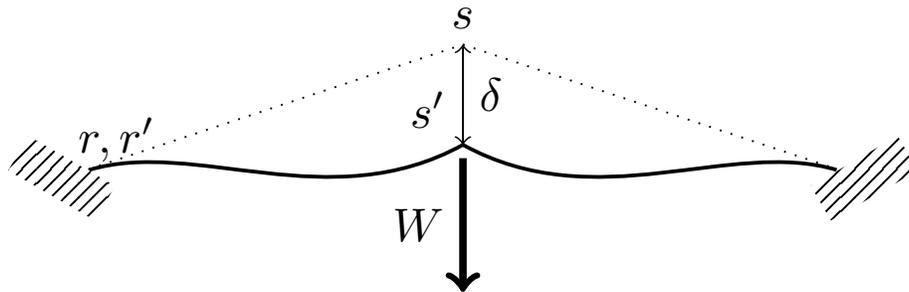
Figure 2.5: Symmetrical Deformation of Toggle, [29]
