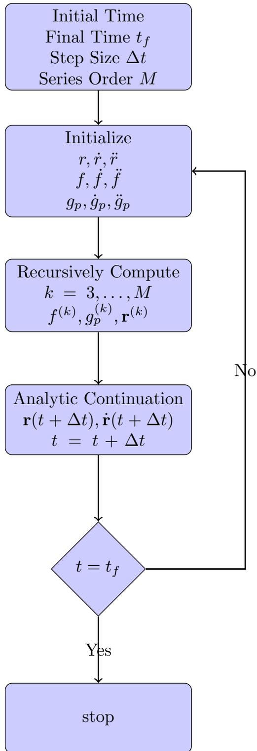
Figure 3.21: The Analytic Continuation Algorithm
