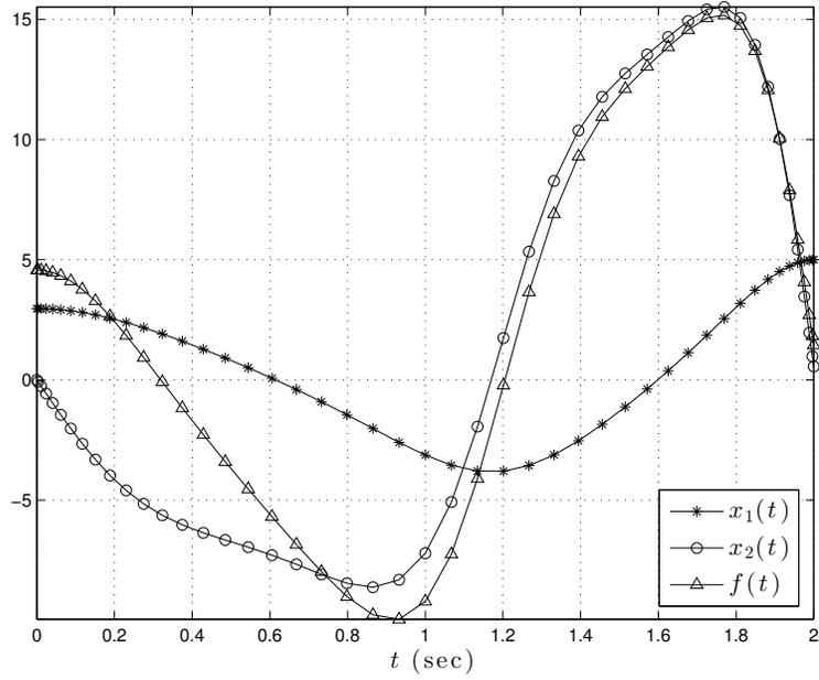
Figure 5.13: States and Controller, Duffing Prescribed Initial Velocity and Final Position, [123]
