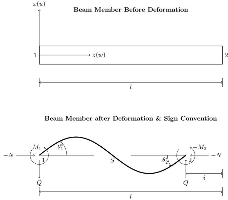
Figure 2.12: Kinematics & Nomenclature for a Beam Member, [29]
