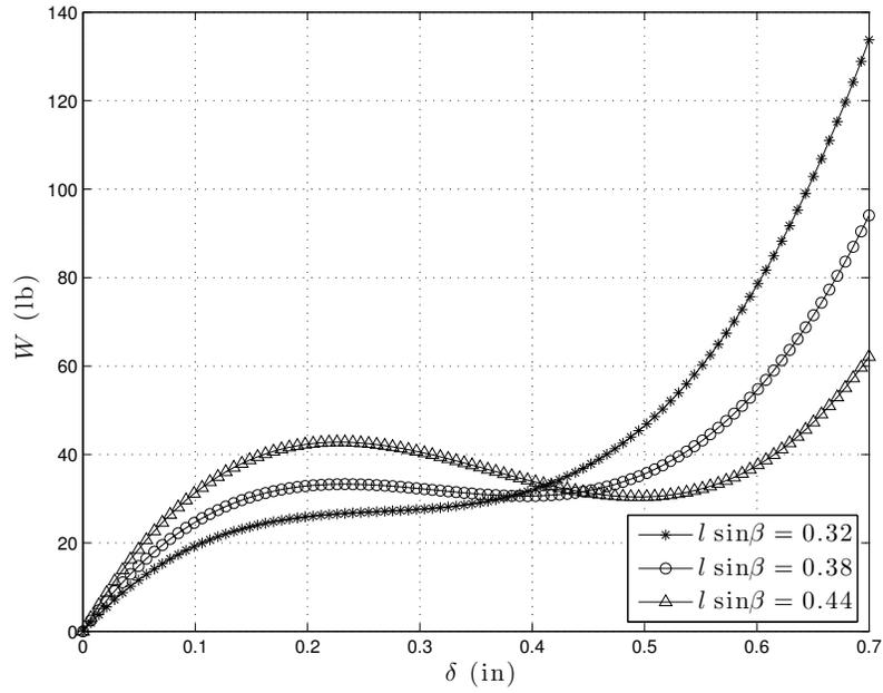
Figure 2.6: Three Cases of Load-Deflection Curves for Williams' Toggle, [29]
