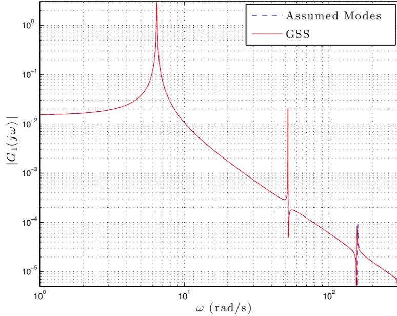
Figure 3.6: Frequency Response Comparison Tip Mass Model at  $x = 4$  ft, [76]
