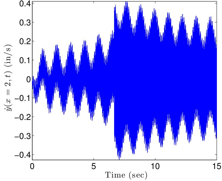
Figure 3.12: Step Input Response  $\dot{y}(x = 2, t)$ , [76]
