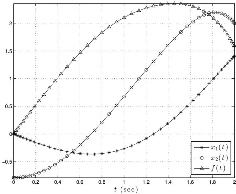
Figure 5.10: States and Controller, Duffing Prescribed Initial Position and Final Velocity, [123]
