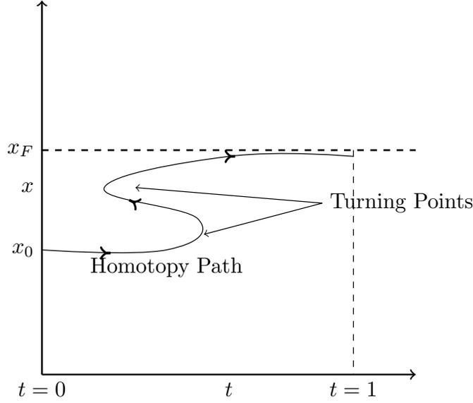
Figure 2.2: Homotopy Path Turning Points
