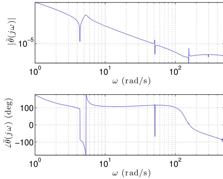
Figure 3.15: Bode Plot  $\bar{\Theta}$ , Designed Gains, [76]
