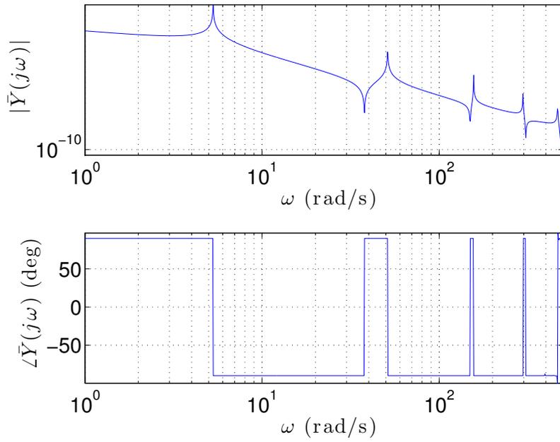
Figure 3.7: Bode Plot  $\bar{Y}$  at  $x = 2$  ft, [76]
