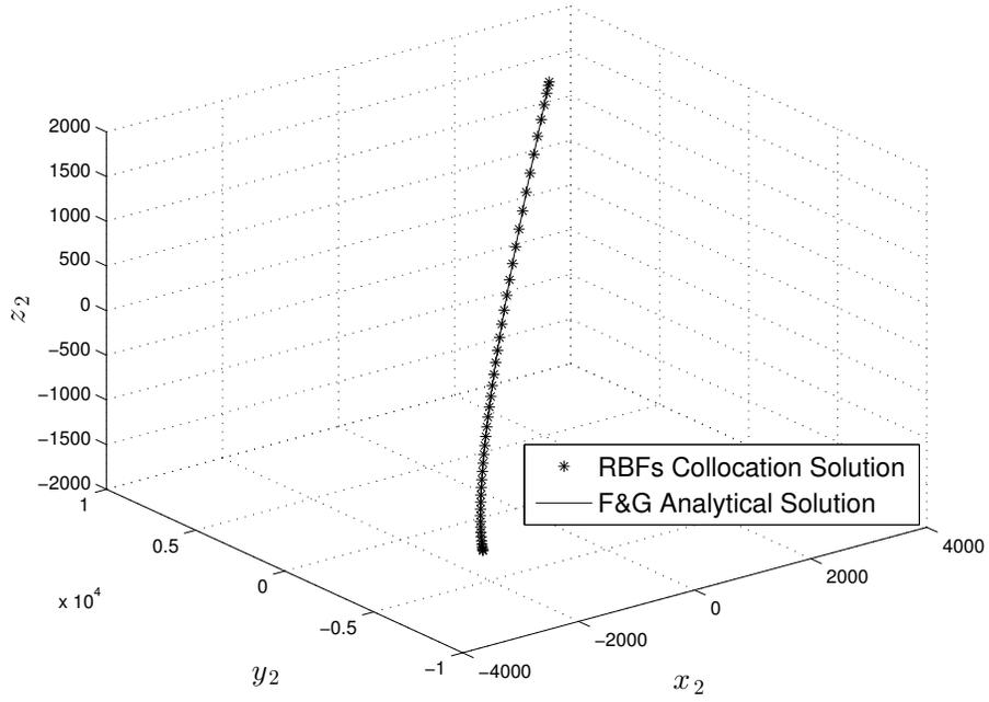
Figure 5.21: Transfer Orbit Velocity Propagation, [123]
