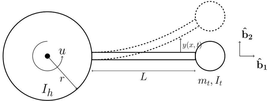
Figure 3.2: Deformation & Axis of Flexible Appendage, [76]
