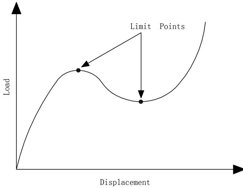
Figure 2.3: Newton's Method Fails at Limit Points, [29]
