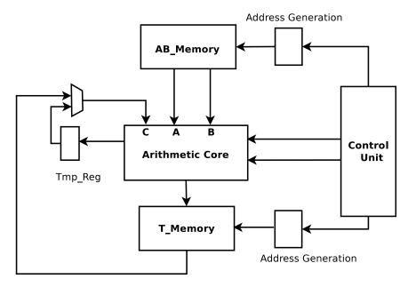
Figure 5.9: Top Level Architecture of the FFAU
