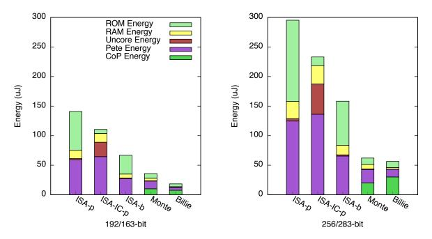
Figure 7.9: Breakdown of energy per Sign + Verify for 192/163- and 256/283-bit key sizes into various sub-components.
