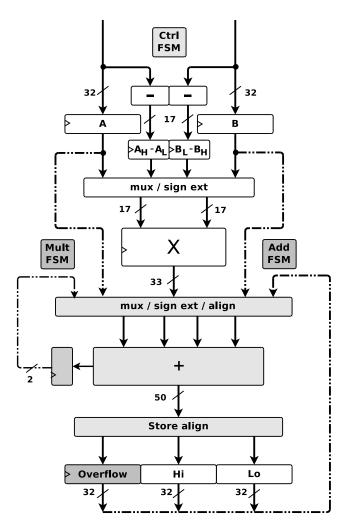
Figure 5.3: The Karatsuba Multiply-Accumulate Unit including support for primefield ISA extensions. The dashed lines represent data paths that have been added or modified to accommodate these ISA extensions. Lightly shaded boxes signify modified components, while darkly shaded boxes indicate additional components.
