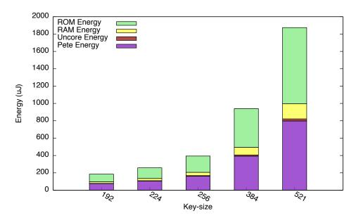
Figure 7.3: Energy per Sign + Verify vs. key size for our baseline with no hardware acceleration.
