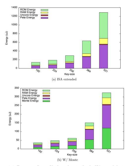
Figure 7.4: Energy per Sign + Verify vs. key size for the ISA extended microarchitecture and the architecture accelerated with Monte.
