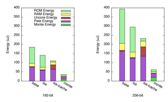
Figure 7.2: Breakdown of energy per Sign + Verify for 192 and 256-bit key sizes into various sub-components.
