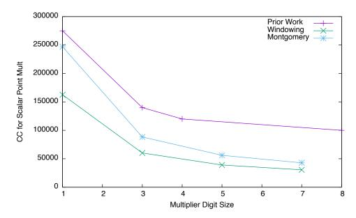
Figure 7.14: Performance for 163-bit scalar point multiply comparing Billie to prior work [42].
