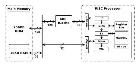
Figure 5.6: Pete with an instruction cache. Notice the interface to the program ROM has been increased to 128-bits.
