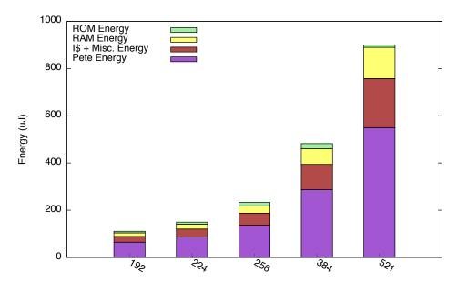
Figure 7.13: Energy per Sign + Verify vs. key size for prime ISA extended microarchitecture with 4KB instruction cache.
