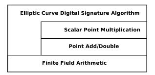
Figure 4.1: Elliptic Curve Digital Signature Algorithm computation hierarchy
