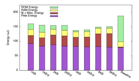
Figure 7.12: Energy per 192-bit Sign + Verify with real instruction cache for various cache configurations. The "-p" indicates the presence of a prefetcher.
