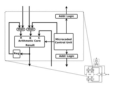
Figure 5.8: The Finite-Field Arithmetic Unit at the center of "Monte"
