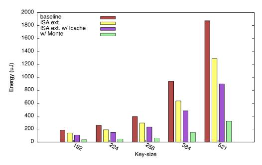
Figure 7.1: Energy per Sign + Verify vs. key size and microarchitecture for prime fields.
