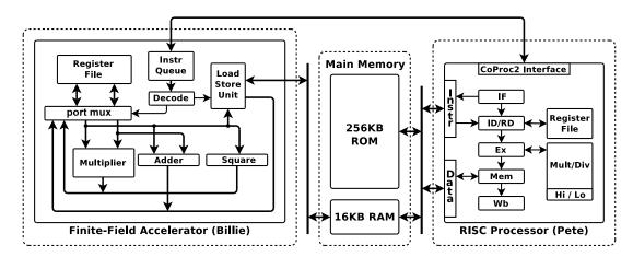
Figure 5.11: The binary-field accelerated architecture, "Pete with Billie"
