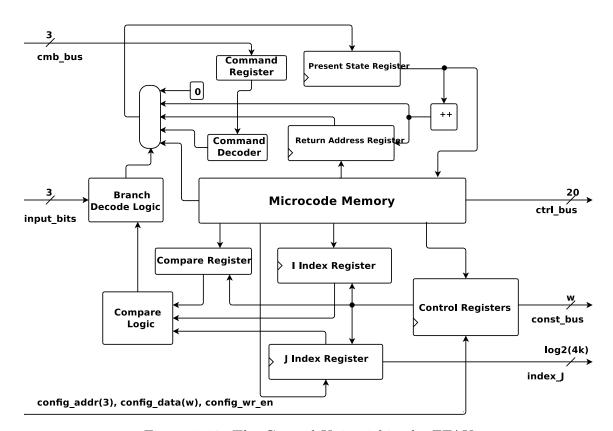
Figure 5.10: The Control Unit within the FFAU
