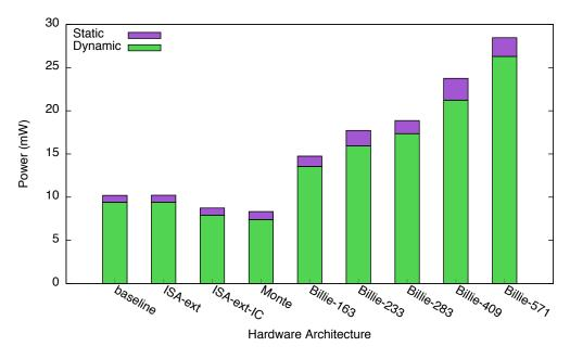
Figure 7.10: Static and dynamic power of evaluated microarchitectures.
