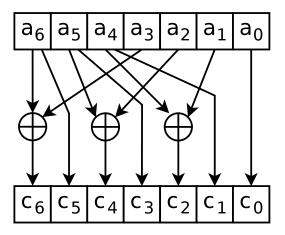
Figure 5.13: Binary-field squaring unit, s.t.  $f(x) = x^7 + x + 1$  [16]
