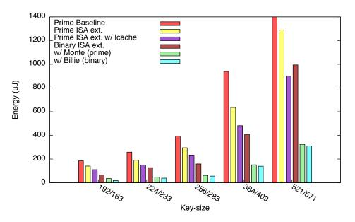
Figure 7.7: Energy per Sign + Verify vs. key size, comparing prime and binary fields of equivalent security.
