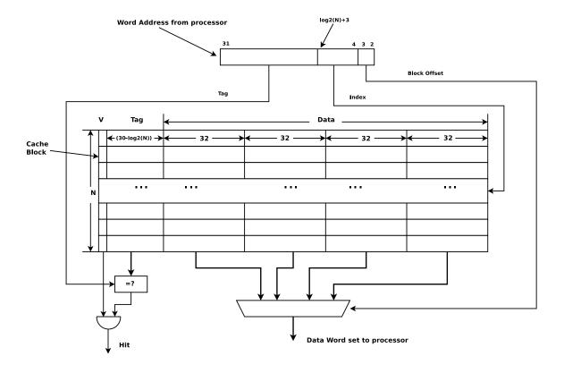
Figure 2.5: A direct-mapped cache with a block size of 16 bytes and a 32-bit word width.
