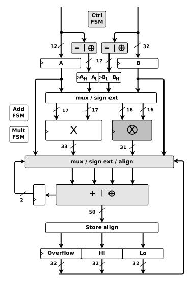
Figure 5.4: The Karatsuba Multiply-Accumulate Unit including support for primeand binary-field ISA extensions. Lightly shaded boxes signify modified components, while darkly shaded boxes indicate additional components.
