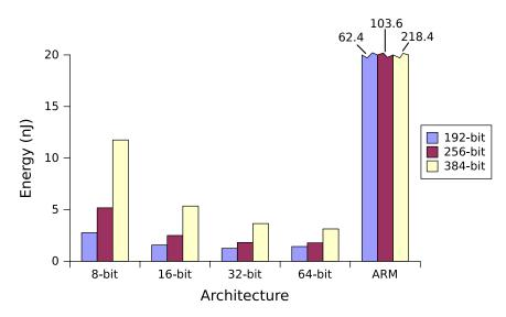
Figure 7.15: Energy per Montgomery multiplication vs. datapath width
