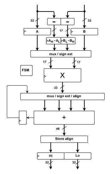
Figure 5.2: The Karatsuba Multiply Unit within the baseline architecture.
