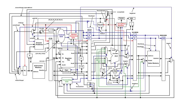
Figure 2.4: The microarchitecture of a 5-stage pipeline processor
