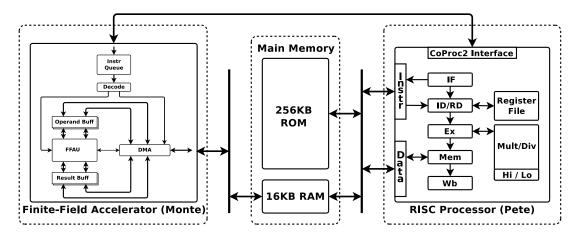
Figure 5.7: The prime field accelerated architecture, "Pete with Monte."
