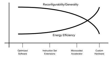
Figure 1.1: The hardware acceleration trade-off.
