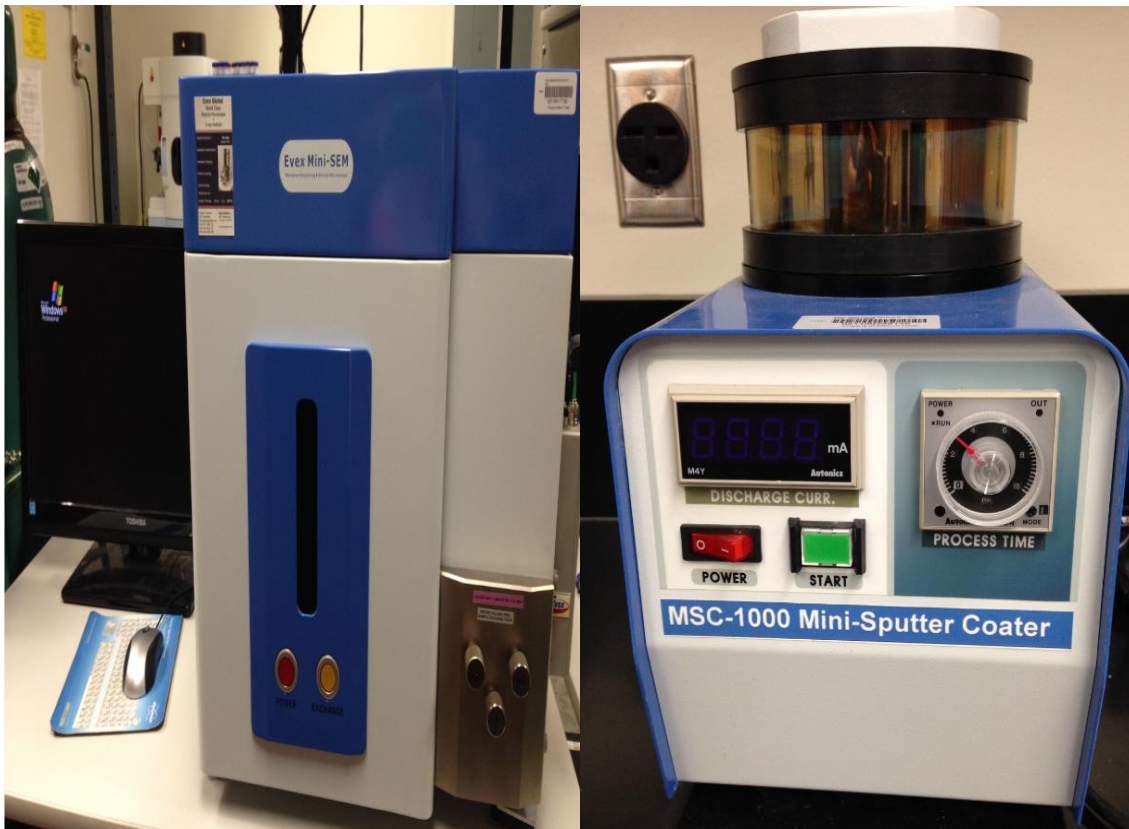
Fig. 20—Evex Mini- Scanning Electron Microscope (SEM) with MSC-1000 Mini-Sputter Coater and energy-dispersive X-ray spectroscopy (EDS).
