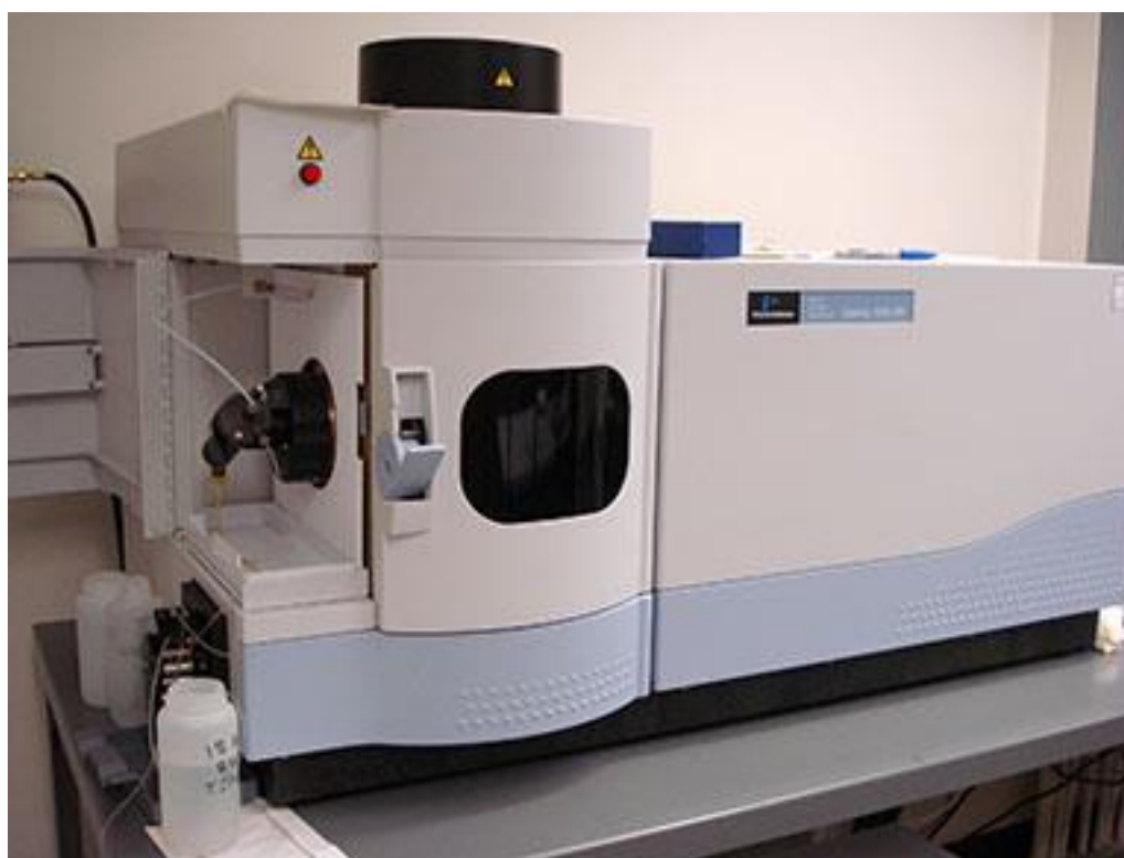
Fig. 17— Optima 7000 DV Inductively Coupled Plasma (ICP).
