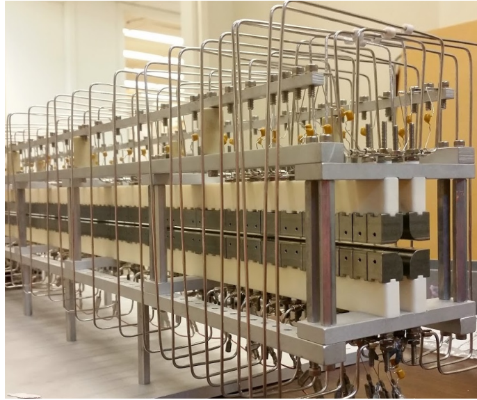
Figure 5.4: A photo of the TAMUTRAP RFQ cooler/buncher during test assembly. The in-vacuum electronic circuitry is visible at top and bottom.
