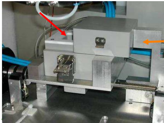
Figure 5. Lead pig used to unload the target disk. The walls of the lead pig are 5.0 cm thick.
