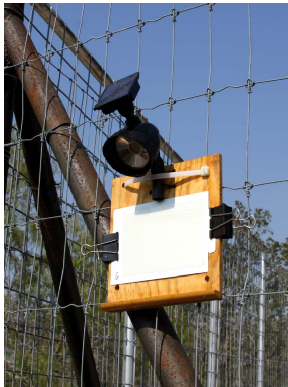
Fig. 1. An insect trap with light source used in the preliminary study. Traps were mounted to the fence around deer pens with zip ties.
