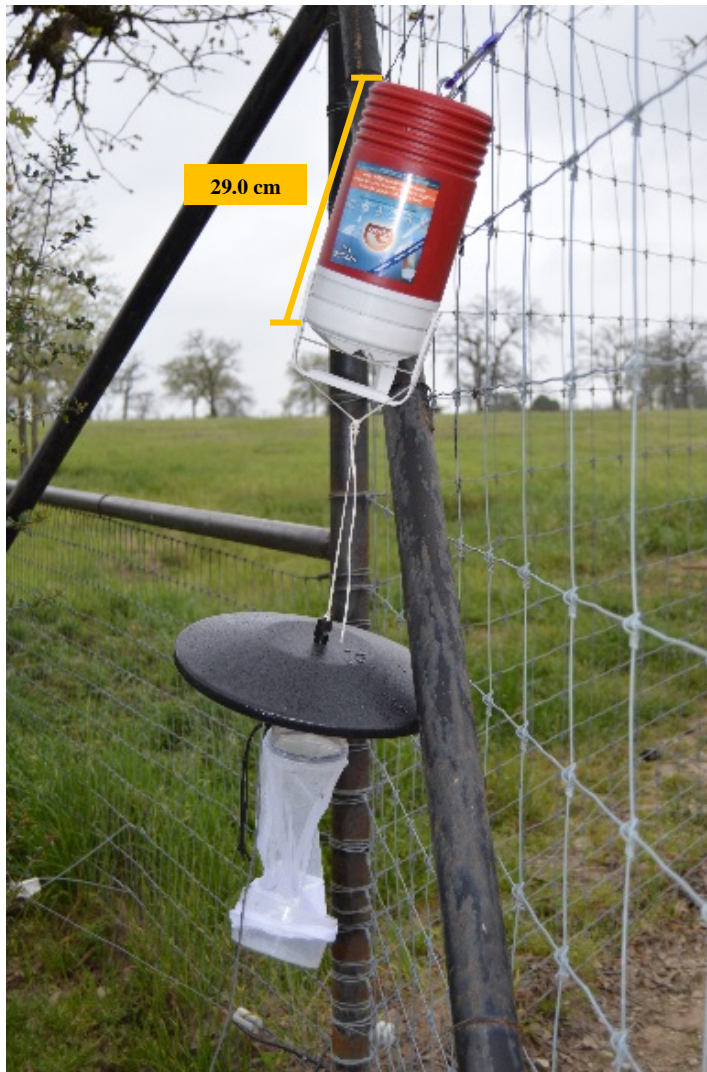
Fig. 30. A photograph of the CO 2 insect trapping equipment. A CO 2 trap was secured to the fence surrounding the deer pens to attract and capture Culicoides spp. overnight.
