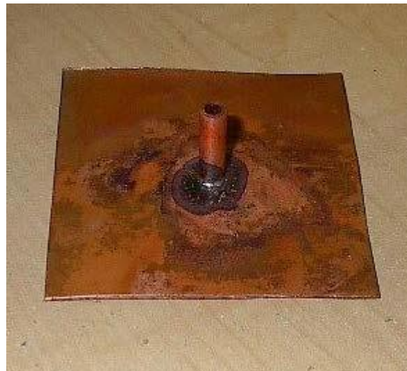
Figure 17. A Well Made Pressure Tap Following Standards
