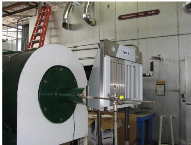
Figure 12. Range Hood Airflow Test Setup
