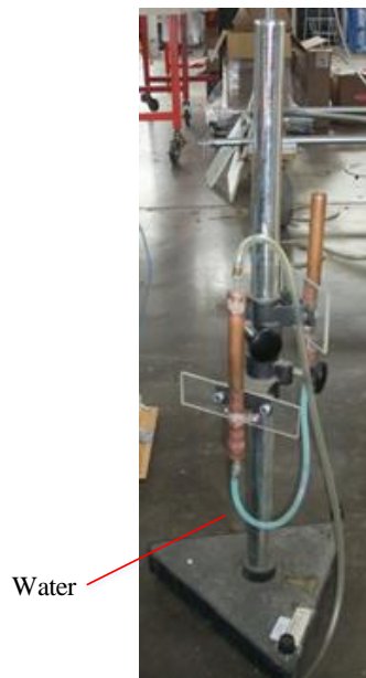
Figure 48. Manometer Used for Reference Pressure Supply
