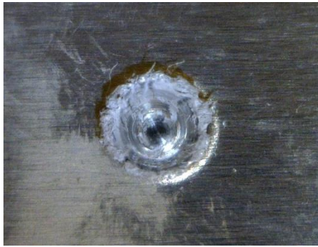
(a) Tool travel 0.08 inch from contact at position A.
