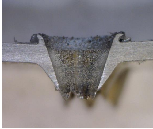
(e) Tool travel 0.235 inch from contact at position D.
