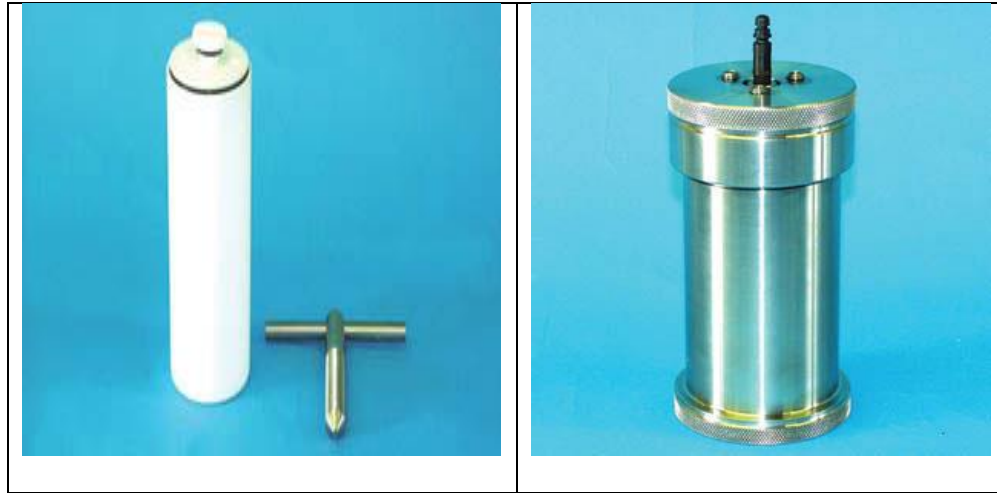
Fig. 4 —Teflon liner and aging cell for thermal stability tests.
