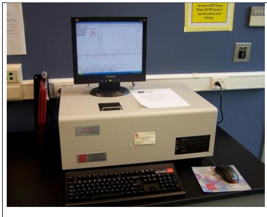
Fig. 5 —The zeta potential indicates the degree of repulsion between adjacent, similarly charged particles in a dispersion
