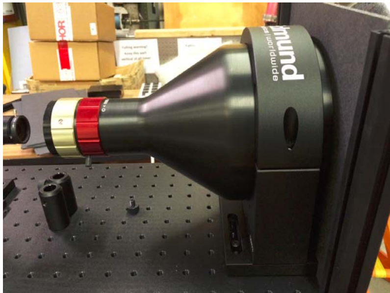
Figure 10 Edmund Optics 0.064X Techspec Gold Series Focusable Telecentric Lens
