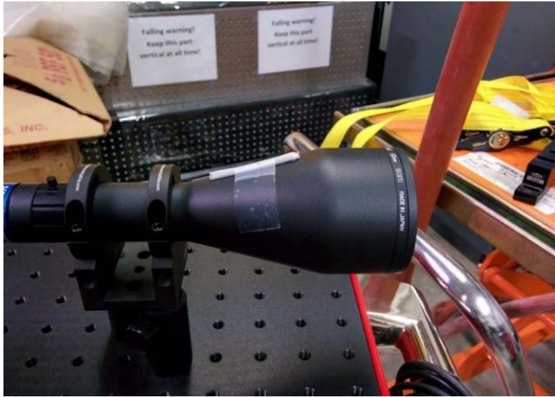
Figure 9 Edmund Optics 0.16X Techspec Silver Series Telecentric Lens
