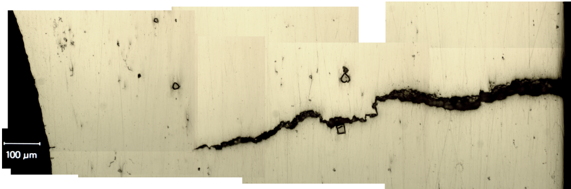
Figure 37: High magnification of the macroscopic crack in L-T plane presented in Figure 36 prior to etching.
