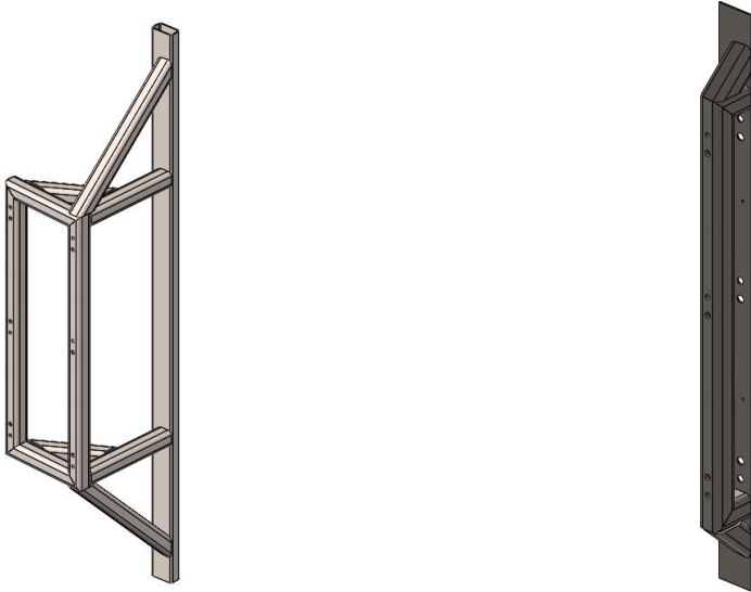
Figure 4.5: Structure 1 and Structure 5 of the diffuser wall panels
