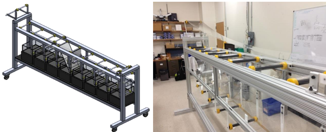
Figure 33. Schematic (left) and picture (right) of pilot scale continuous LbL coating apparatus.
