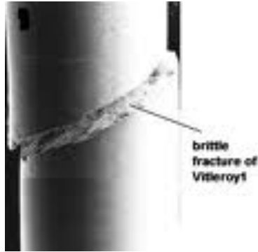
Figure 2: Scanning electron micrograph of brittle MGs failed after tension
