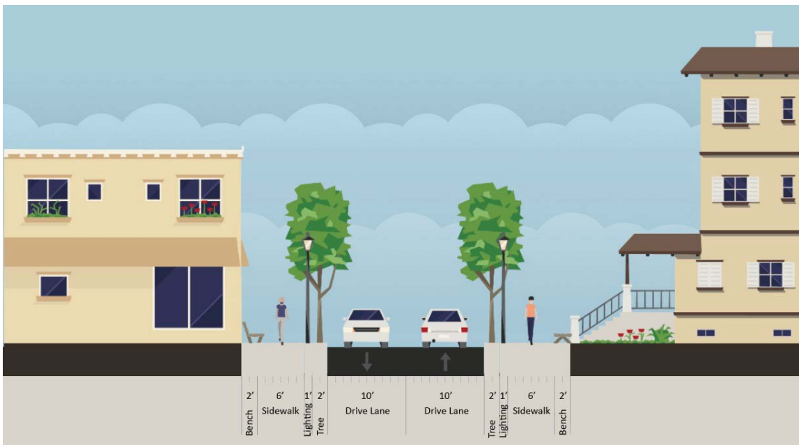
Figure 4-12 Cross Section for Local Street
