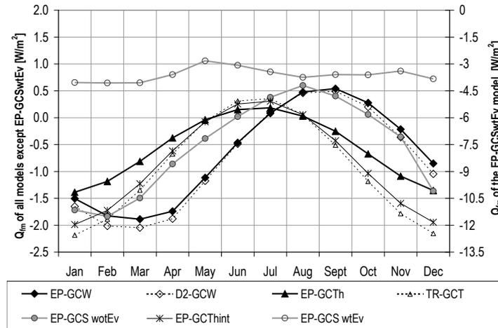
**Figure 1.** Monthly average floor heat fluxes of the Austin sealed box.
