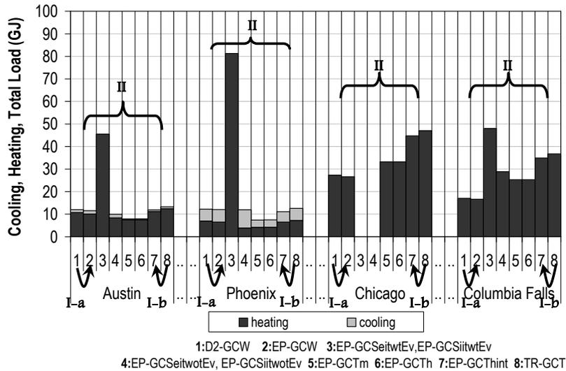
**Figure 5.** Cooling, heating and total thermal loads of the sealed boxes.
