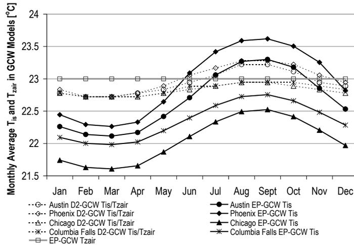
**Figure 6.** Monthly average inside surface temperatures ( $T_{\text{is}}$ ) and zone air temperatures ( $T_{\text{zair}}$ ) of the Winkelmann floors of the sealed boxes.
