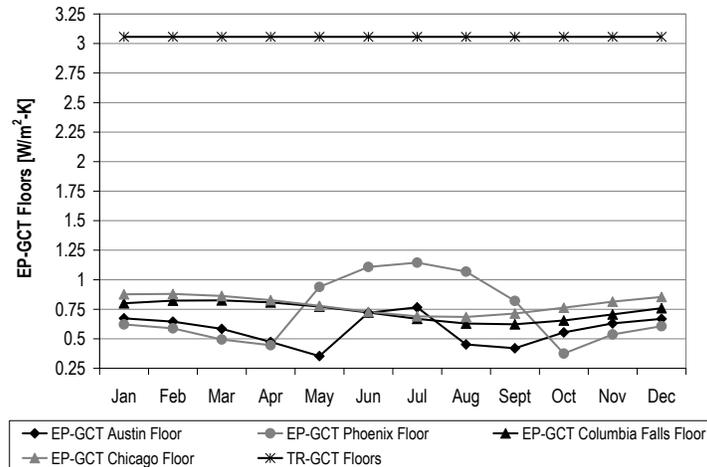
**Figure 8.** The convection coefficients of the *TRNSYS* floors.
