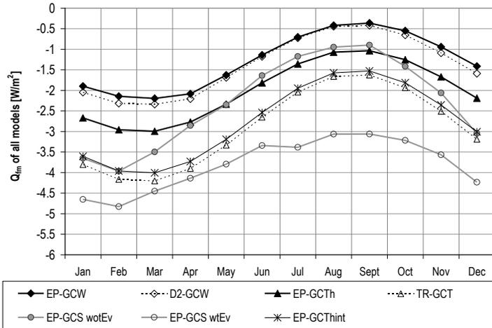
**Figure 4.** Monthly average floor heat fluxes of the Columbia Falls sealed box.
