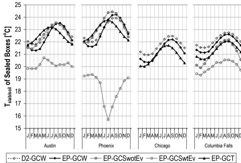
**Figure 7.** The slab-soil interface temperatures ( $T_{\text{slab/soil}}$ ) of the sealed boxes.
