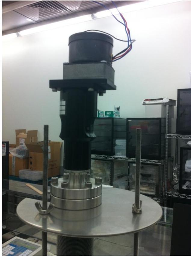
**FIG. 10.** AC 10rpm Motor
