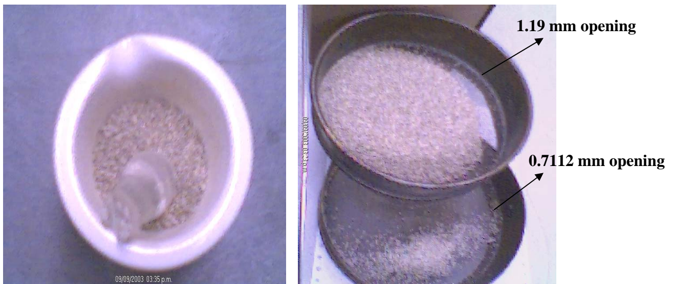
Fig. 2.9 – Reduction of size of organoclay particle in laboratory.
