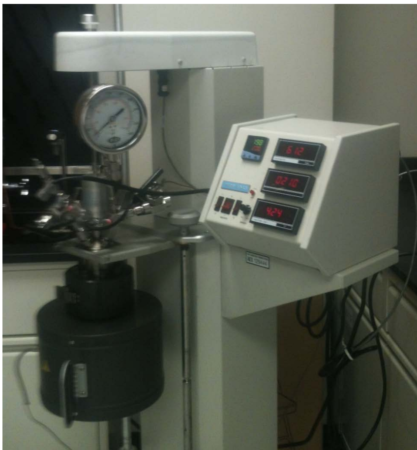
Figure 3: The continuously mixed high temperature and high pressure reactor . (4570-Parr Instrument, Moline, IL, USA)
