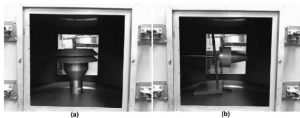
FIG. 4. Photos showing the (a) \text{PM}_{10} and (b) isokinetic inlet in the same sampling planes.
