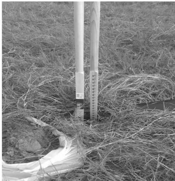
Figure 1. Soil is removed from hole and placed into plastic garbage bags in order of removal so that horizons can be replaced in order.
