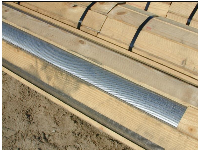
Figure 25. Antelope Hills pre-packed screen. Reprinted from Jehn-Dellaport (2013).
