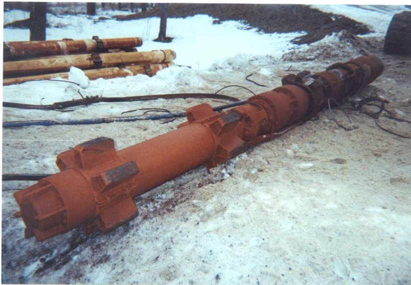
Figure 23. Submersible pump used for a horizontal well along the Raccoon River, Des Moines Iowa. Reprinted from Rash (2013).
