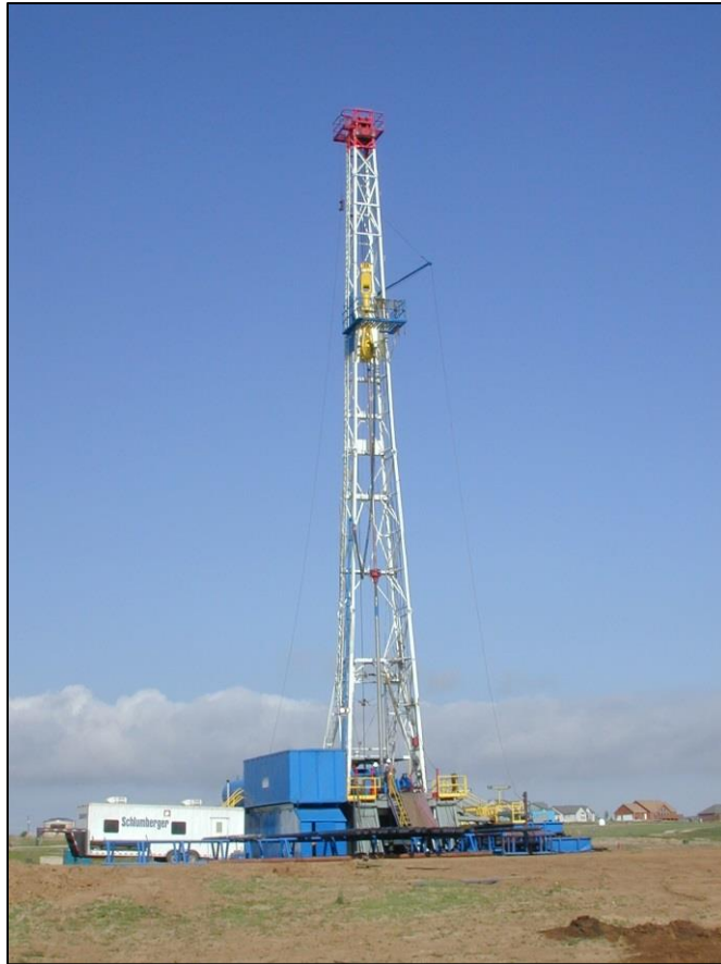
Figure 26. Antelope Hills directional groundwater well rig. Reprinted from Jehn-Dellaport (2013).
