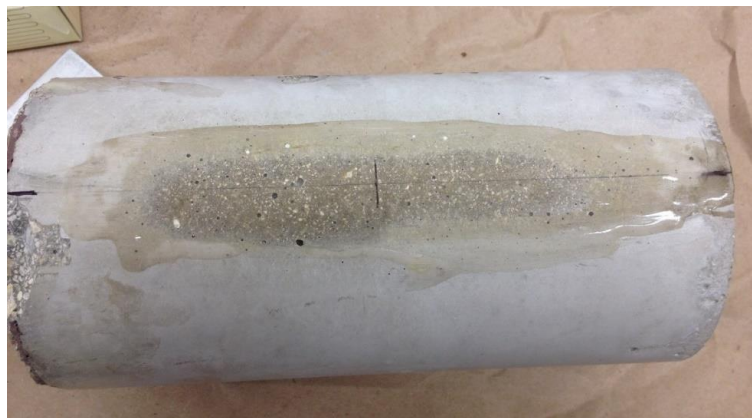
Figure 3.23. Concrete Cylinder Ready for Gaging.
