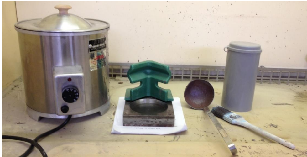
(a) Sulfur capping equipment
