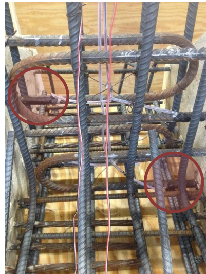
(b) Strain gages on bars
