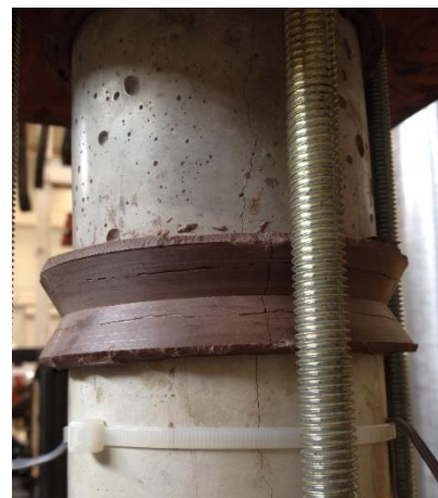
(b) Opposite face cracked
