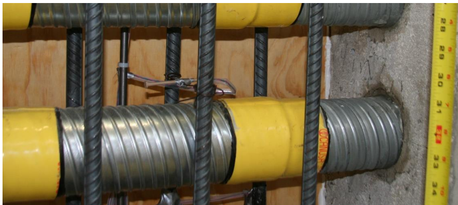
(c) Embedded concrete gage in the splice
