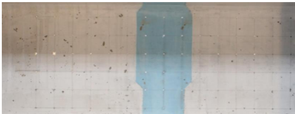
(e) DEMEC Points on the south side of the specimen
