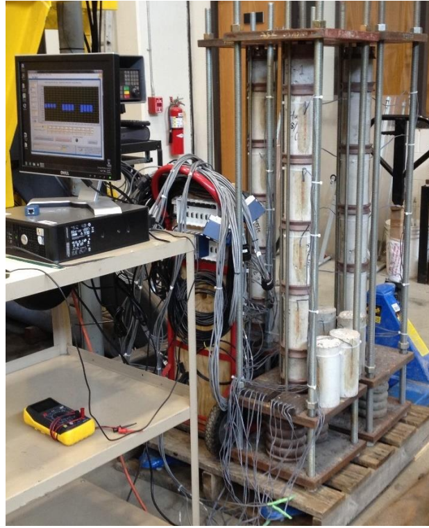
(b) Creep frames loaded and recording data
