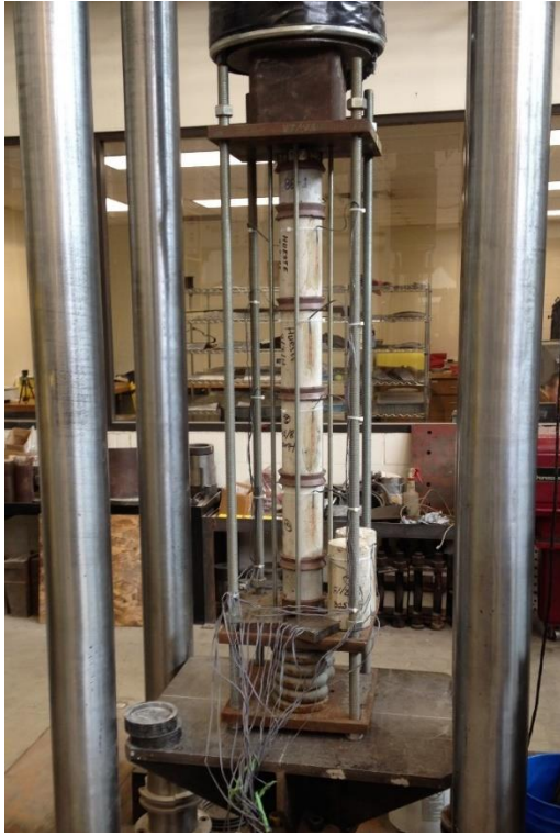
(a) Loading the creep frame
