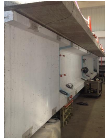
(c) Surface strain gages on top and bottom flanges
