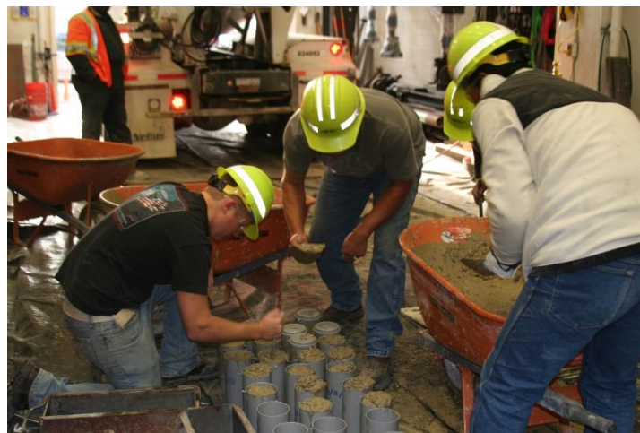
(b) Preparing concrete cylinders and beams
