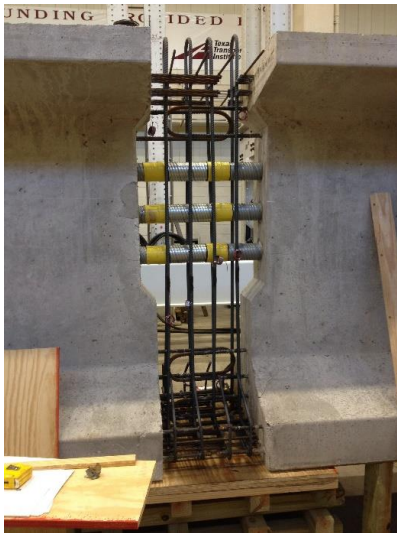
(a) Reinforcement in the splice
