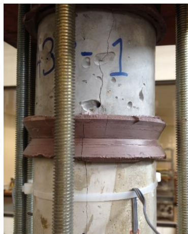
(a) Cracked face of the top half cylinder
