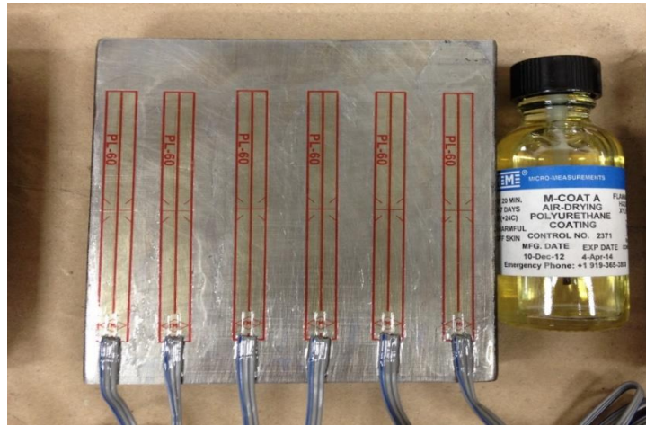
Figure 3.22. One Gaged Steel Plate.
