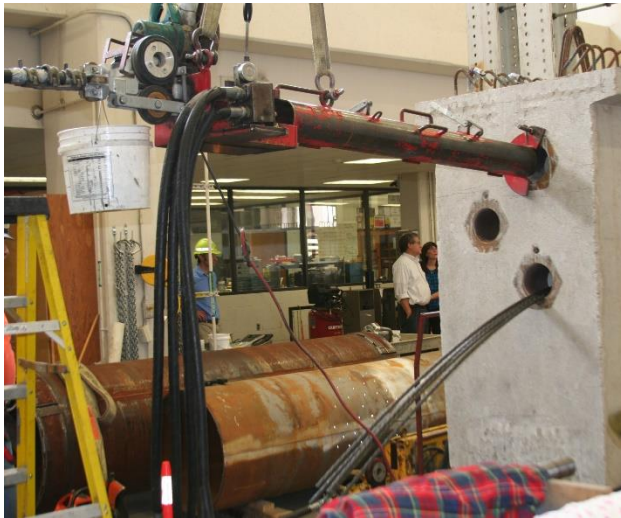
(c) Running strands in top duct
