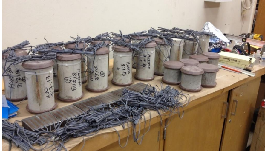
Figure 3.24. Cylinders and Plates, Gaged and Coated.
