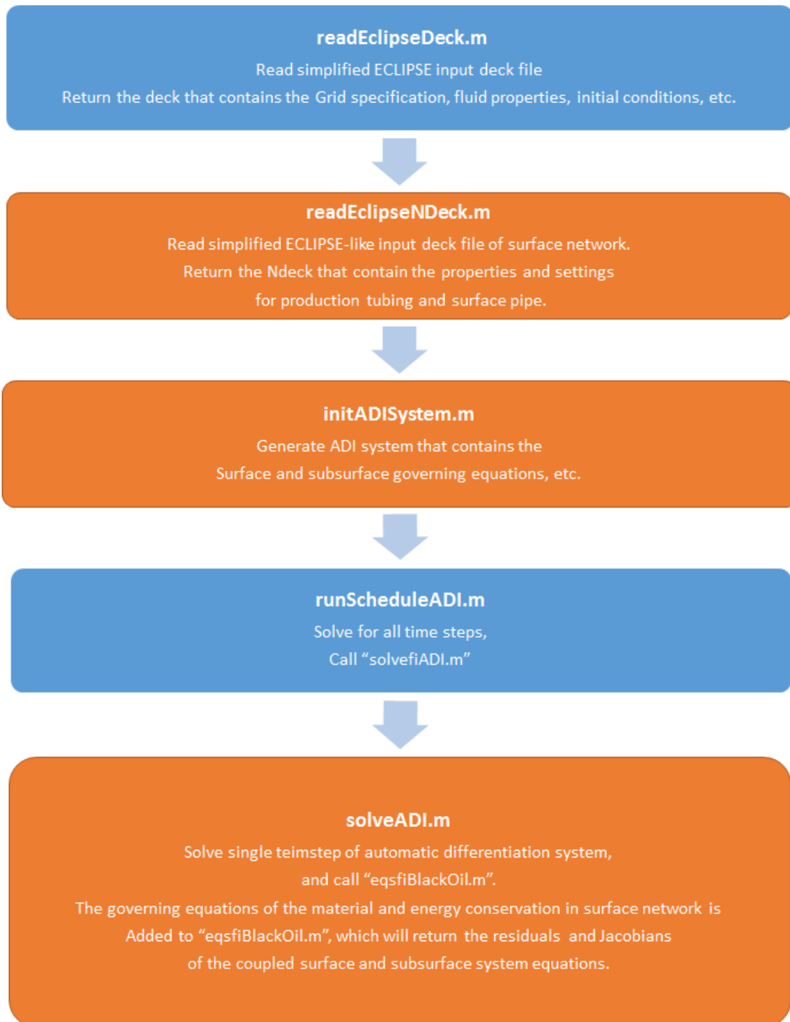
Figure 5.2: General procedure of modified MRST fully implicit solver for coupled model
