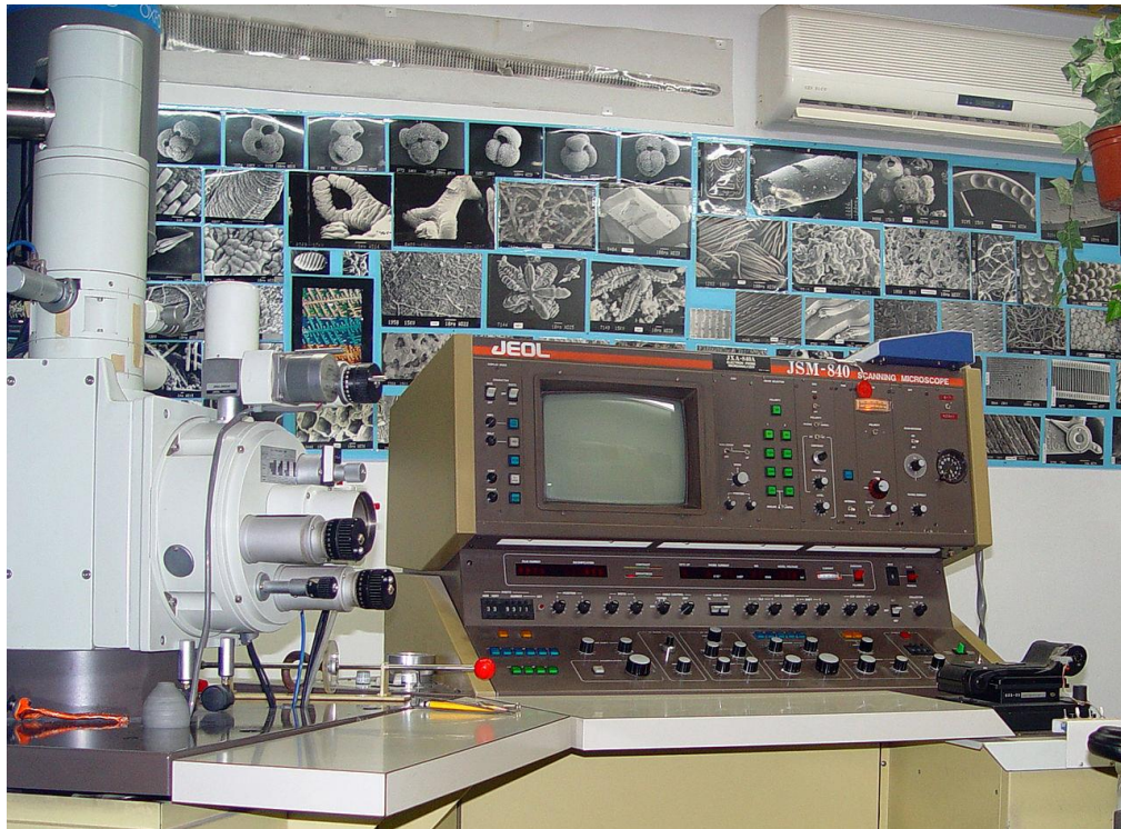
Figure 5. Analog type scanning electron microscope in the Geological Survey of Israel Laboratory [8]
