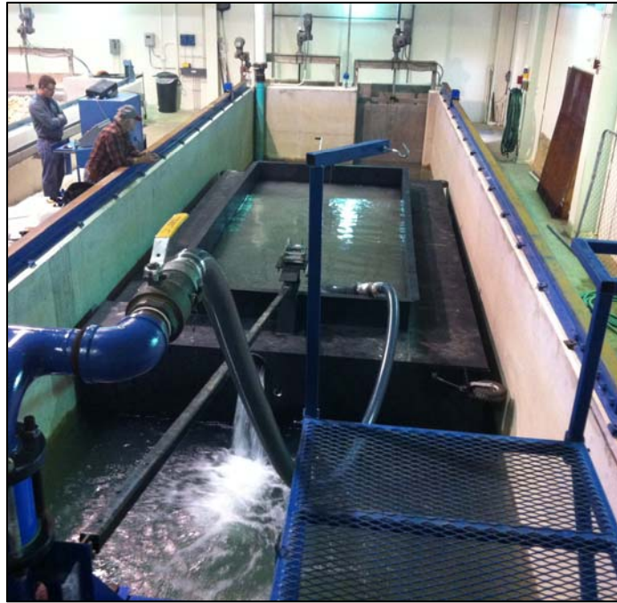
Figure C - 4: Discharge pipe and hopper barge during dredge testing.
