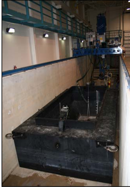
Figure C - 1: Empty hopper barge prior to testing.
