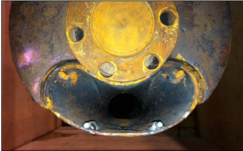
Figure C - 14: Dredge suction mouth with bolts attached.
