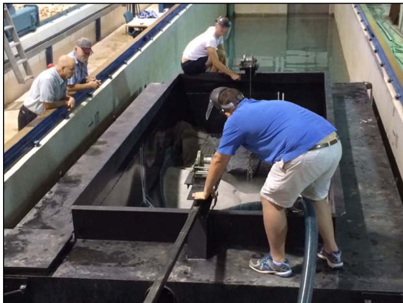
Figure C - 7: Emptying sand from hopper barge after a day's tests.
