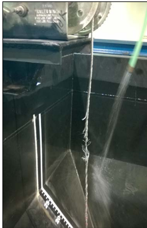
Figure C - 9: Failed cable on hopper barge due to overloading on day two of testing.
