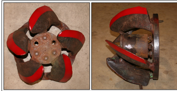
Figure 2: Model cutter head used at the Haynes Coastal Engineering Laboratory.
