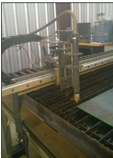
Figure C - 10: Plasma cutter used to construct screens.
