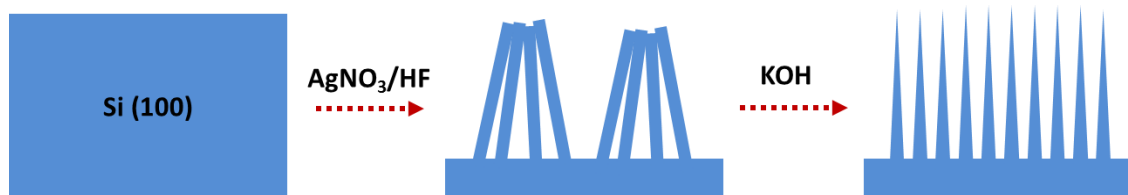
Figure 4.2. Schematic illustration of electroless etching of Si wafers using \text{AgNO}_3/\text{HF} , and KOH solution.
