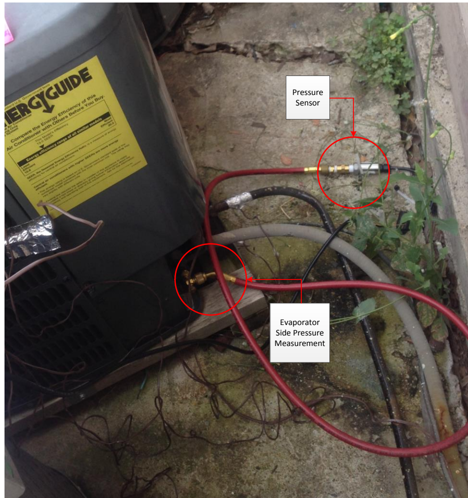
Figure 34: Mounting of the Pressure Sensor for Evaporator Pressure Measurement
