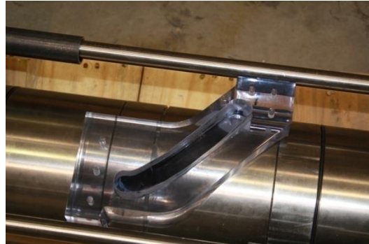
Figure 3-12: Window on the first and second stage of the pump
