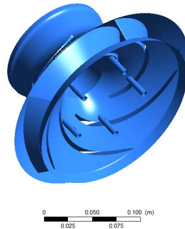
Figure 3-26: ESP impeller and balance holes
