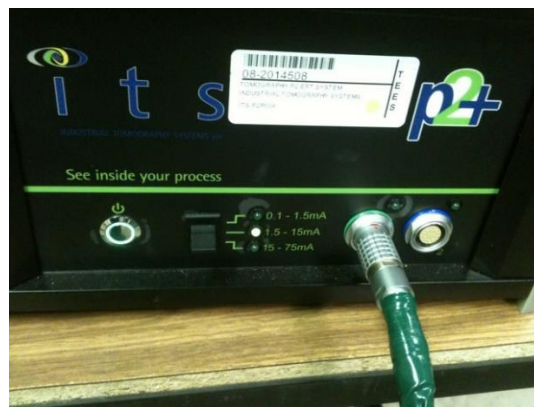
Figure 3-13: Industrial Tomography Systems Plc (its) electronic box for conductivity measurements
