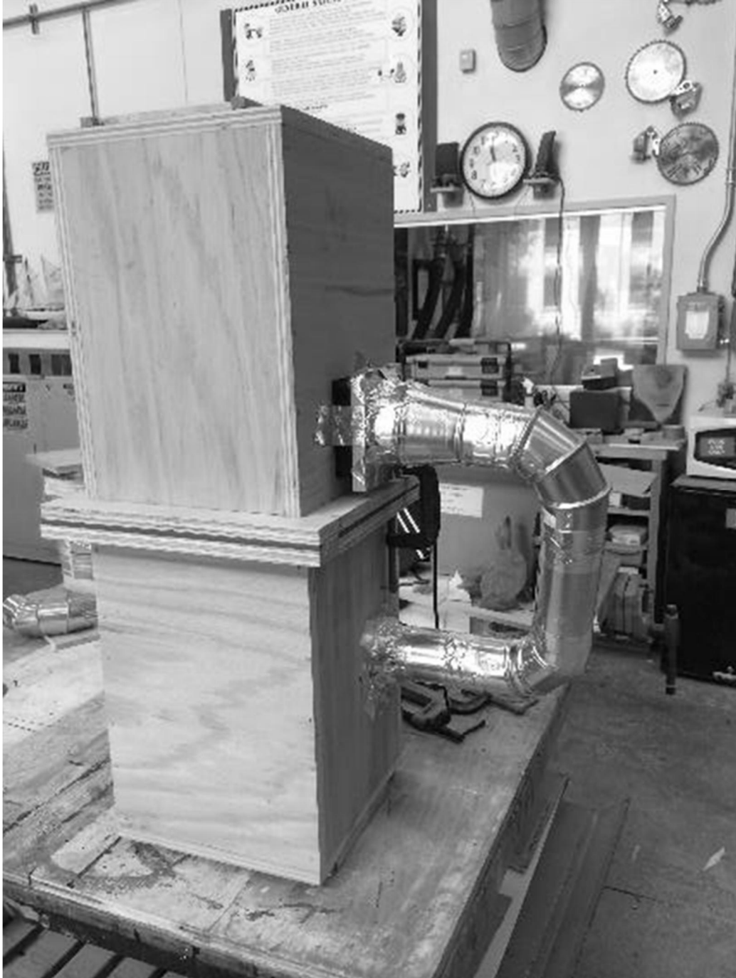
Figure 23. Fan and Duct System
