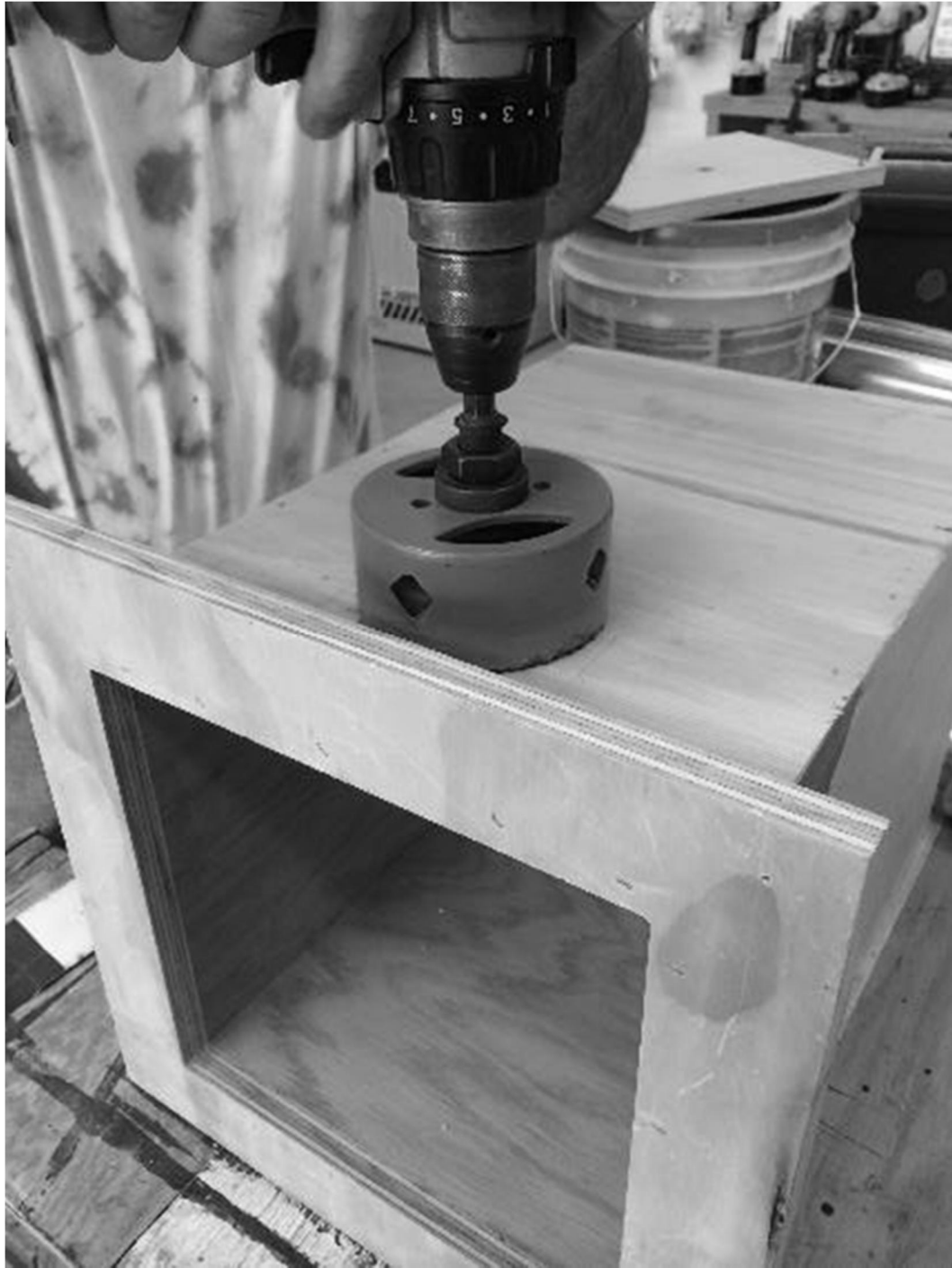
Figure 20. Drilling a Hole in the Containment Vessel for the Fan
