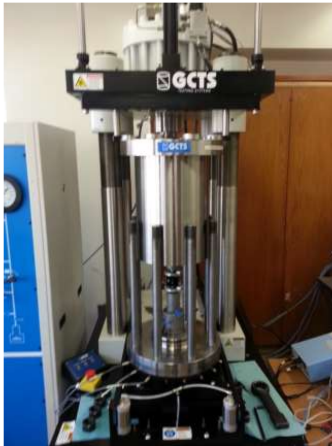
Figure 7 - Open triaxial cell with sample in place
