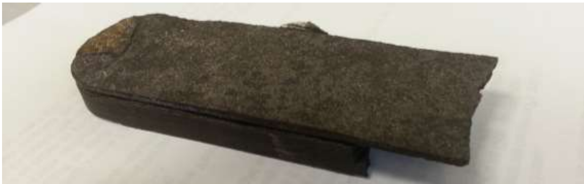
Figure 28 - FL3 fracture surface
