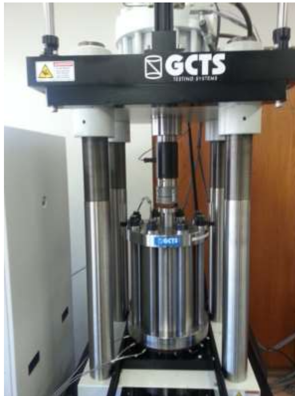
Figure 11 - Sealed triaxial cell ready to receive axial load
