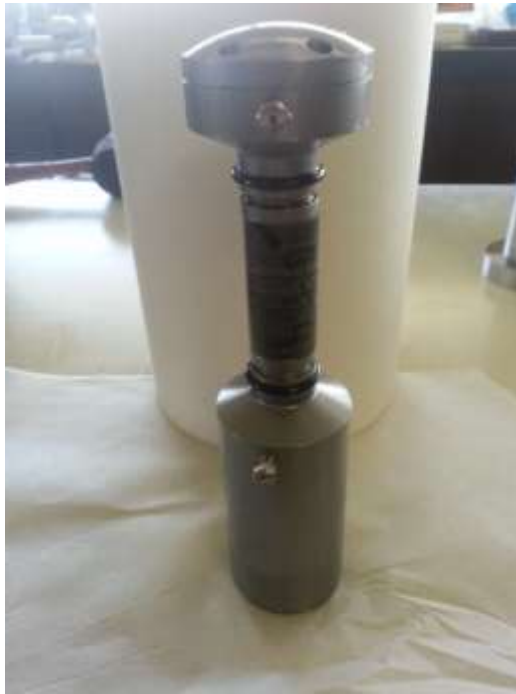
Figure 4 - Eagle Ford core in position between the two platens
