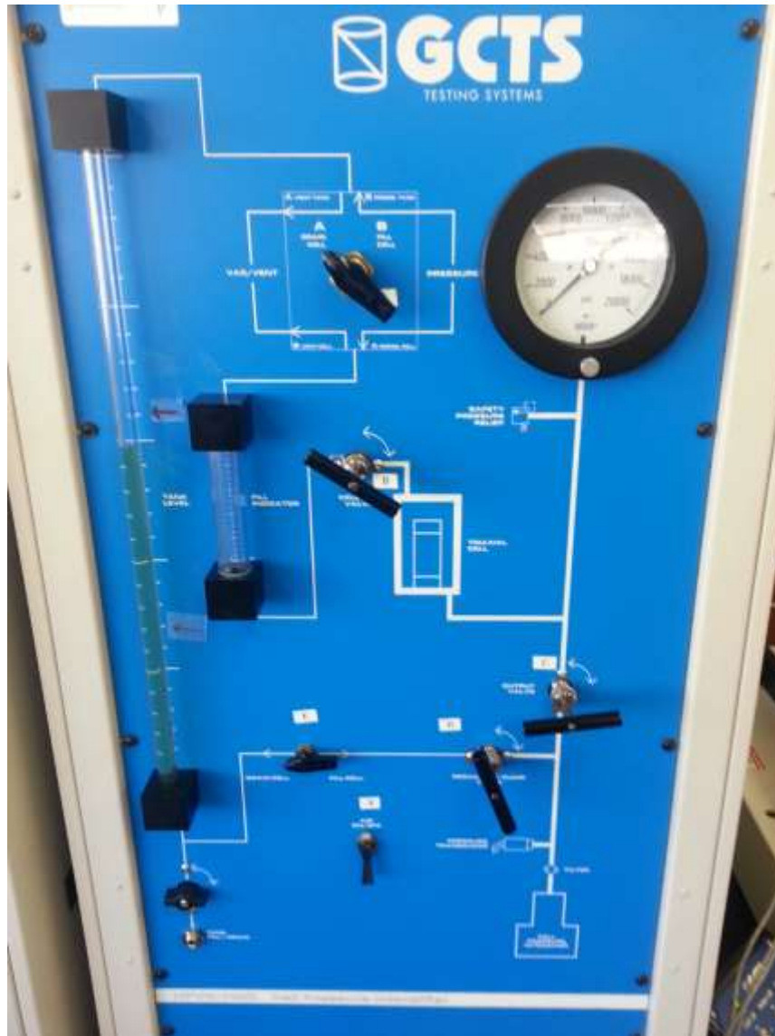
Figure 9 - Cell pressure cabinet with valves for oil control
