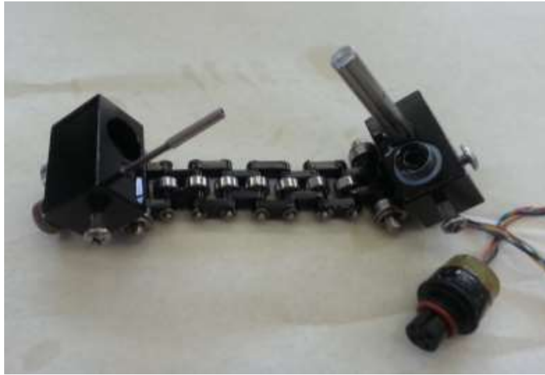
Figure 6 - Chain gauge for measuring circumferential deformation of rock samples
