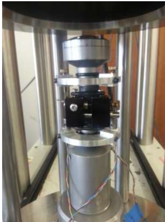
Figure 5 - Rock sample with deformation instrumentation mounted in triaxial cell
