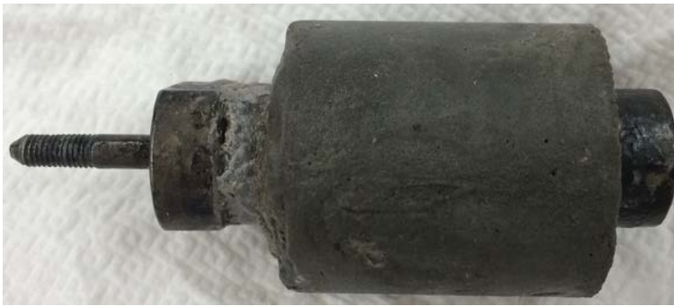
Figure 17: Sample I-A, No Cracks
