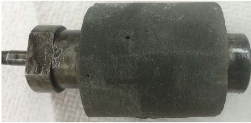
Figure 28: Sample VI-A, Propagating Radial Crack
