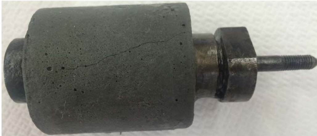
Figure 26: Sample V-A, Single Radial Crack
