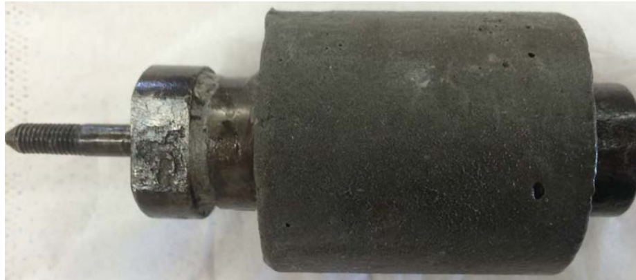
Figure 30: Sample I-B, No Cracks
