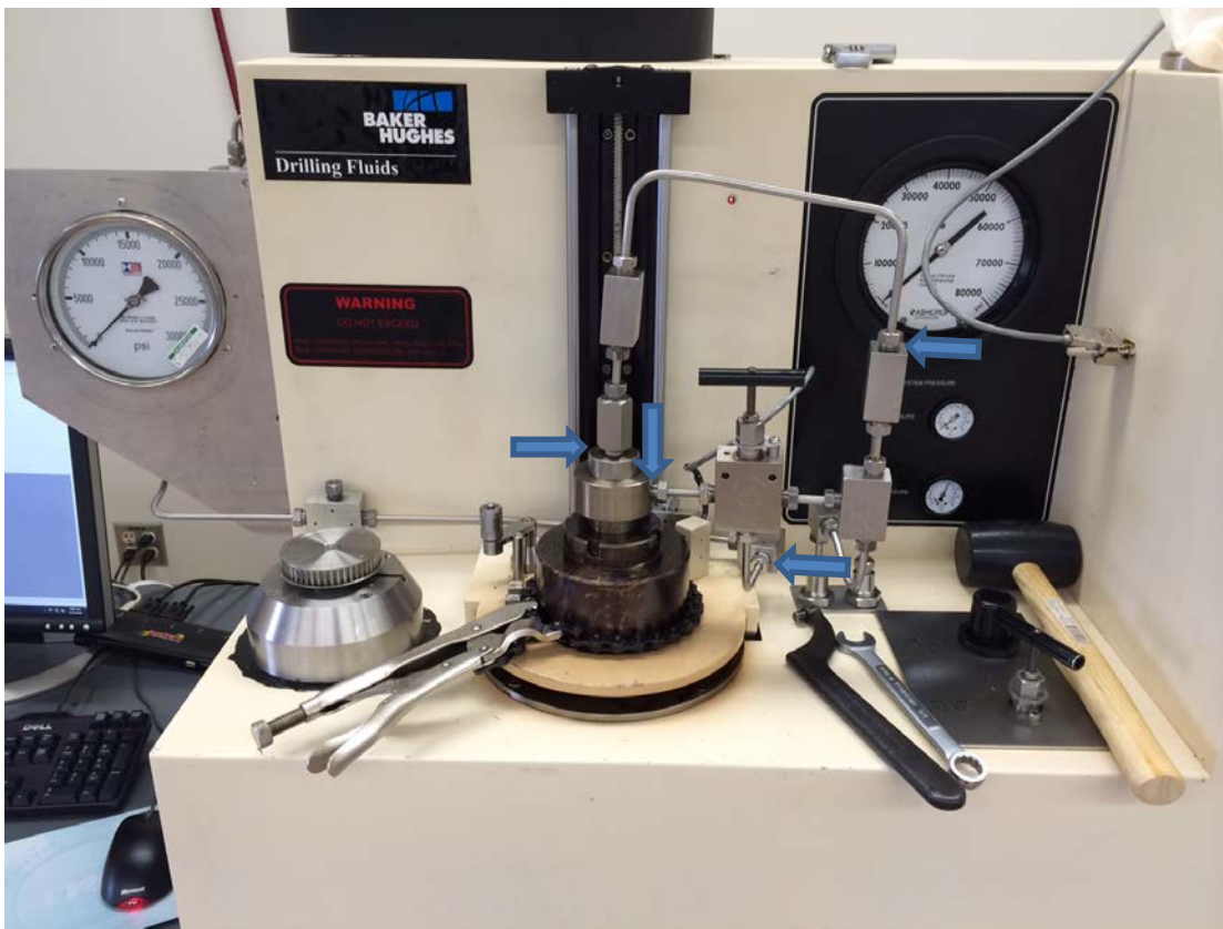
Figure 38: Common Leak Points in HPHT Cell Setup
