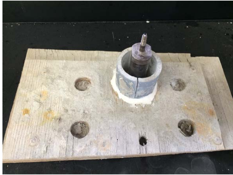
Figure 9: Cement Sheath Mold
