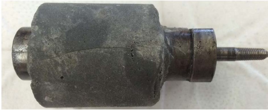
Figure 32: Sample II-B, Single Radial Crack and Disking
