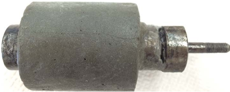
Figure 24: Sample IV-A, Single Radial Crack
