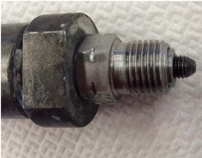
Figure 11: Cell Glands and Collar: Correct Positioning
