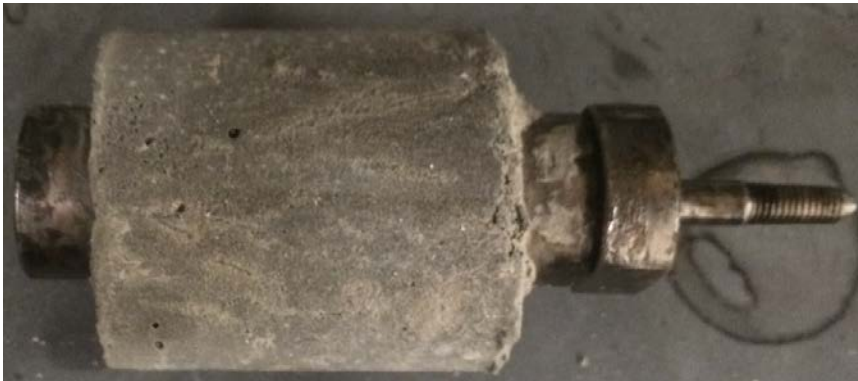
Figure 20: Sample III-A, No Cracks
