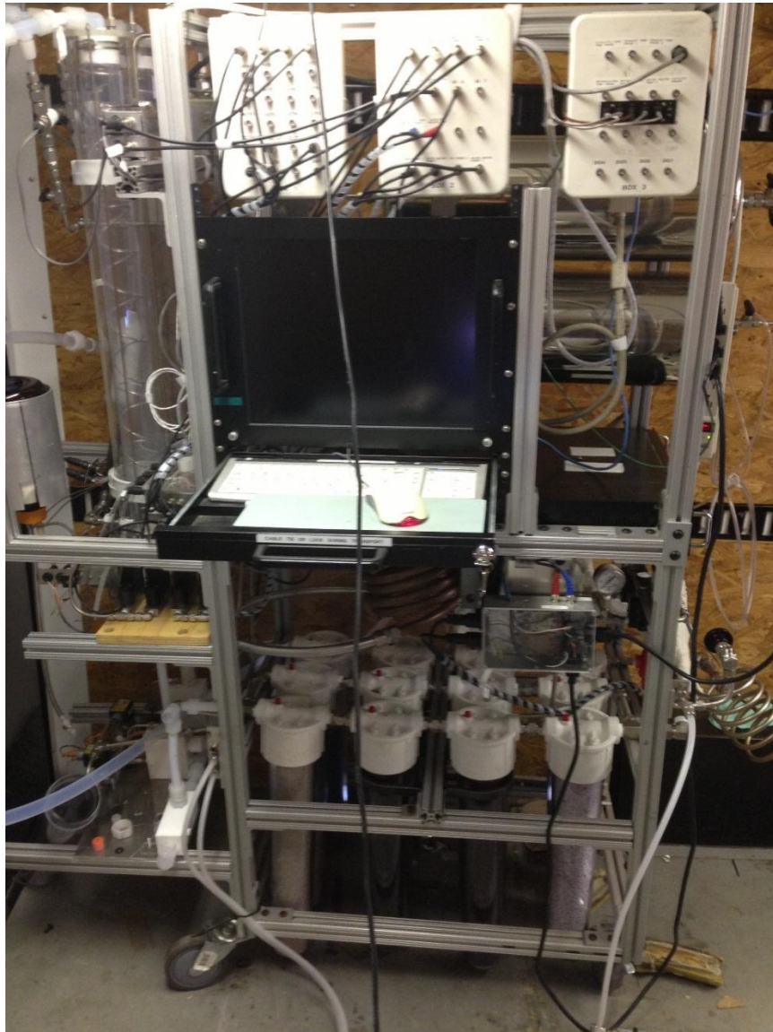
Figure 23. Gas conditioning cart inside the instrumentation trailer.
