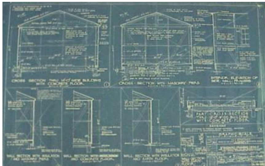
Figure 32 1942 Paint Booth Framing Details
