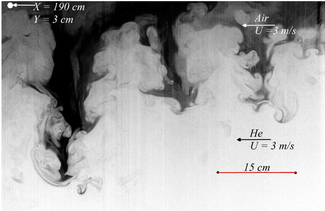
Figure 3.3: Typical instantaneous image taken at x = 150 \text{ cm} , during an experiment with Atwood number 0.75, and U = 3 \text{ m/s} .
