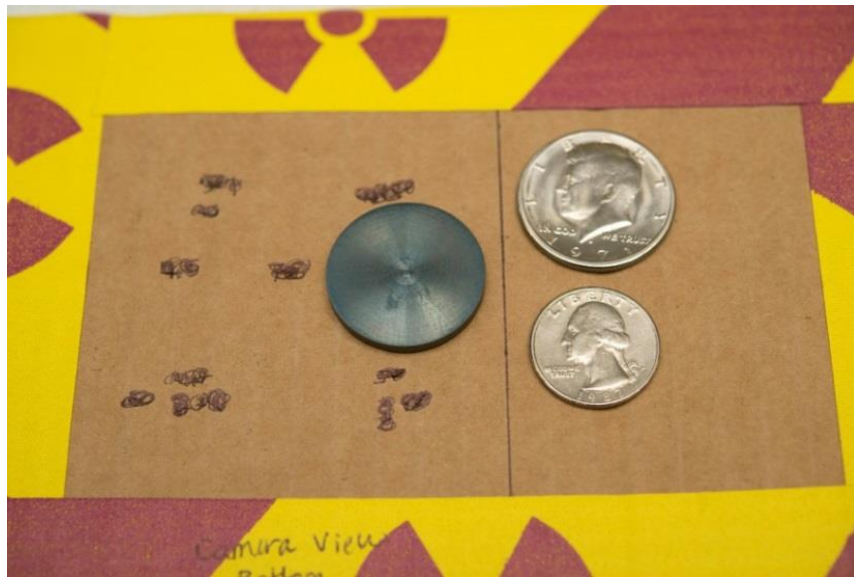
Figure 6. Photograph of U metal specimen next to half silver dollar and quarter.
