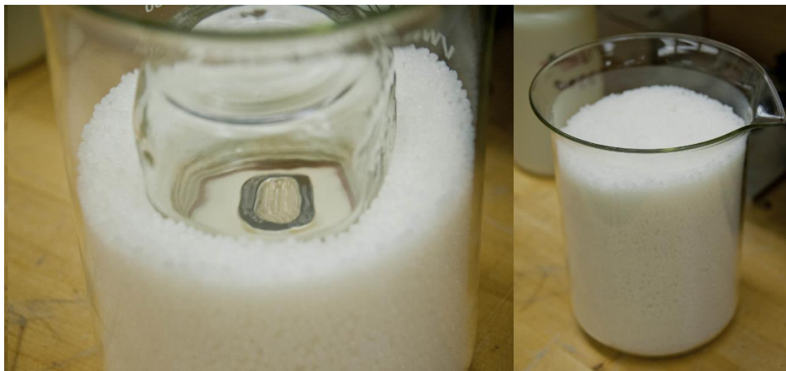
Figure 40. Photograph of ^{210}\text{Po} source surrounded by polyethylene beads.
