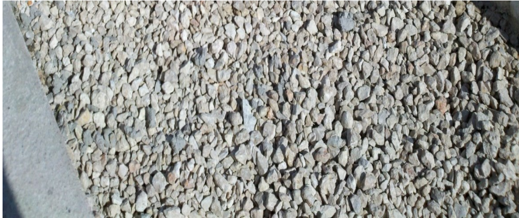
Figure 18 Open Graded Granular Subbase Used for Test Program.
