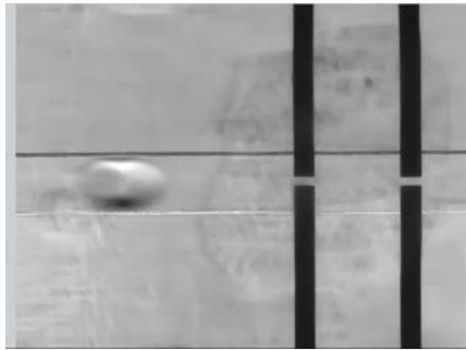
Figure 27: A droplet passing the differential electrodes.
