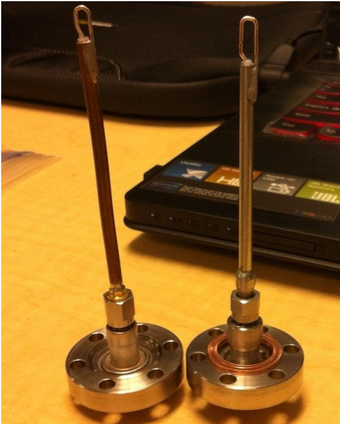
Figure 29: Loop Couplers Made From Semi-Rigid Coaxial Line and SMA to SMA Vacuum Feed-Throughs
