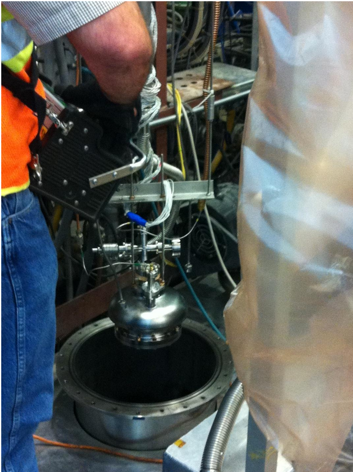
Figure 22: Dewar 1 Test Stand With Wafer Test Cavity Attached at the Base Being Lowered into Dewar
