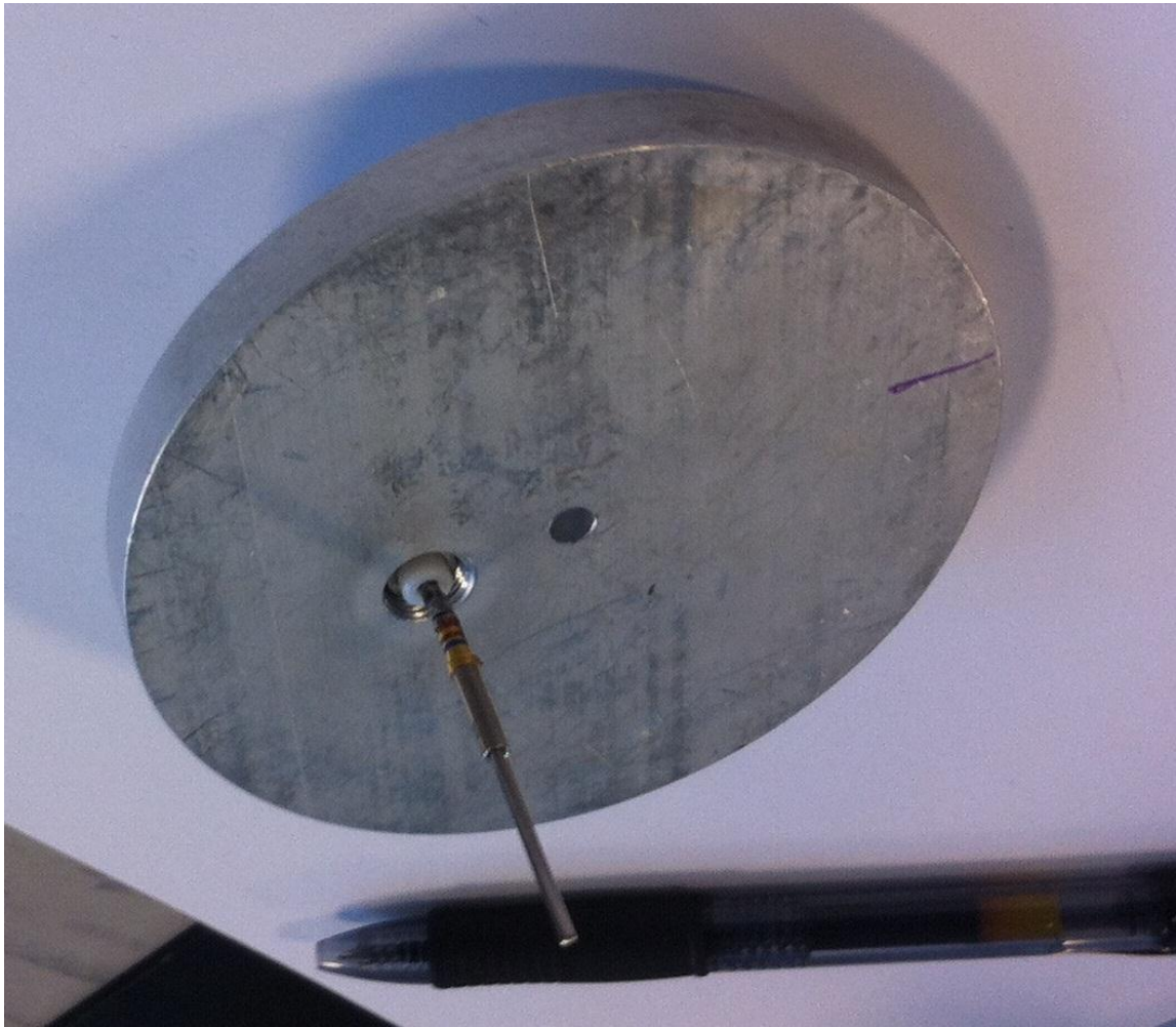
Figure 21: Aluminum Flange With Adapter For Using Welding Rod Antennas
