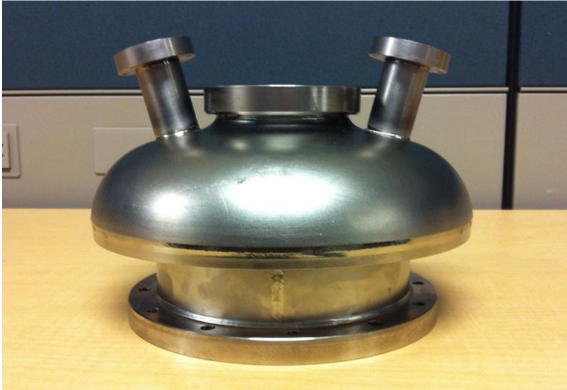
Figure 19: Completed Body Section of the Wafer Test Cavity with Niobium Main Components and NbTi Flanges
