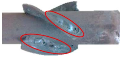
Figure 29 – Rough welding seams of the pre-existing helix-vane swirler
