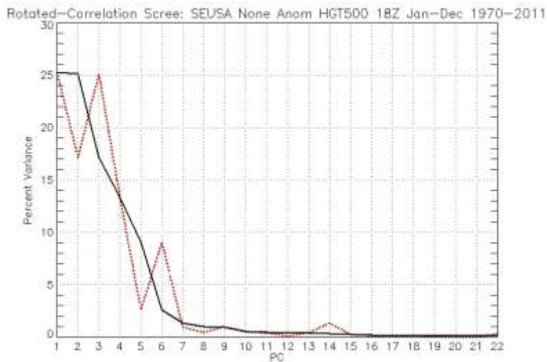
Figure 27. Scree plot with PCs sorted by largest percentage of variance explained (black line) and unsorted variance (red line).
