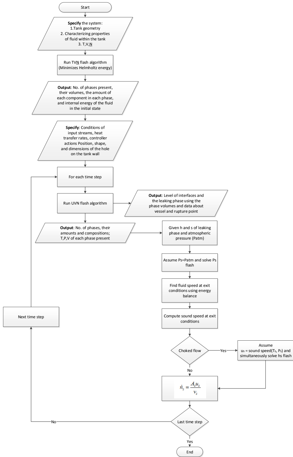
Figure 1: Flow of calculations in the code developed
