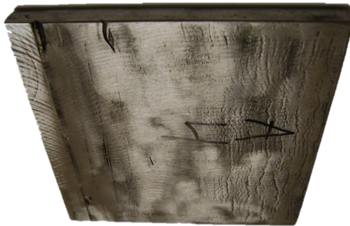
Figure 22. Photograph of AZ31B plate with multiple top surface cracks after ECAE processing. Punch face is on the left and extrusion direction is to the right.
