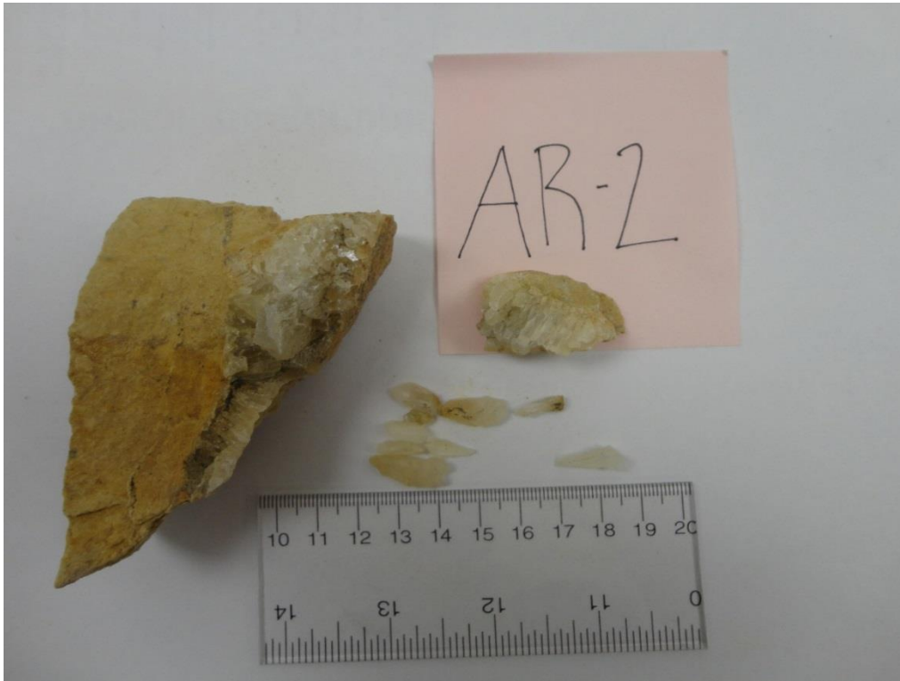
Fig. A-6. Image of sample AR2 collected from modern dissolution veins that cross cut the Bird Spring Formation. Macro-calcite crystals formed in the vugs were collected and analyzed.
