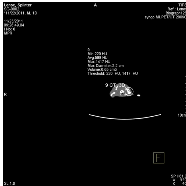
Figure 4-20. Pre PEG impregnation analysis of bone. Initial bone average and range of HU values for Splinter before PEG impregnation were measured using 3D image processing software.
