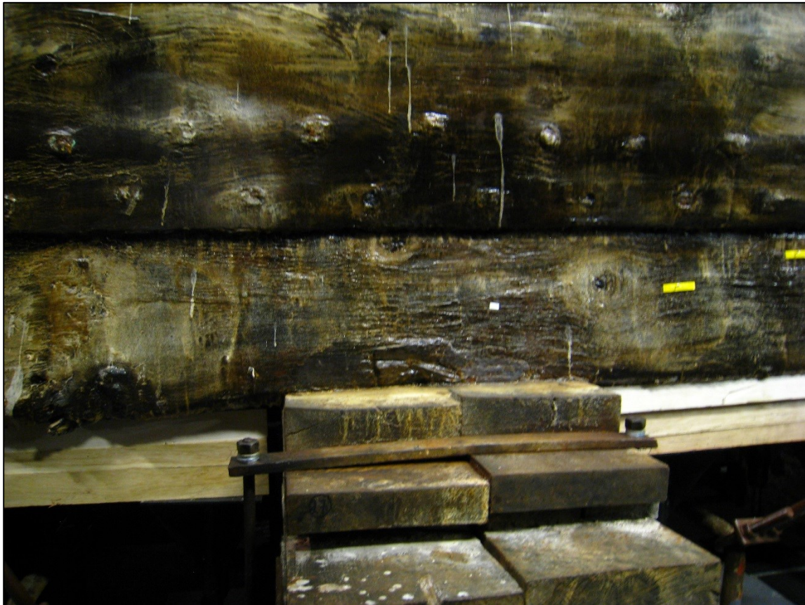
Figure 6.16. Example of crushing distortion of Vasa's keel, on the starboard side near the stem.
