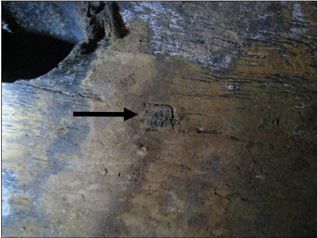
Figure 3.5. Spijkerpen as observed on the inner face of one of Vasa 's removed planks. Photograph by Kelby Rose.
